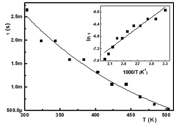
Fig. 6. Temperature dependence of the relaxation time of Al/p-ZnGa<sub>2</sub>Se<sub>4</sub>/n-Si/Al HJD. Inset:  $\ln \tau$  versus  $1000/T$ .
