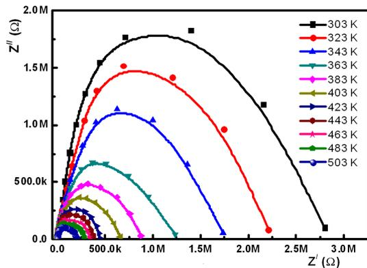
Fig. 5. Cole-Cole plots of Al/p-ZnGa<sub>2</sub>Se<sub>4</sub>/n-Si/Al HJD.
