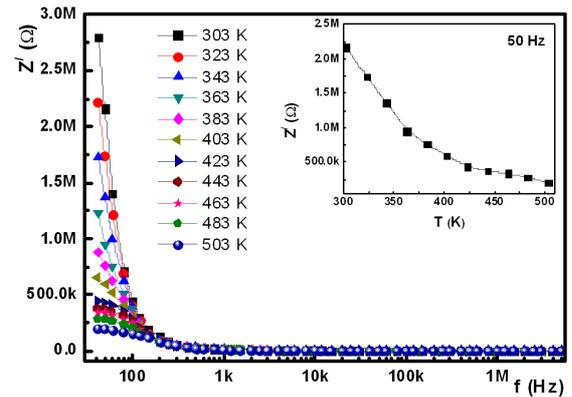
Fig. 2. Frequency dependence of the real part of impedance  $Z'$  at different temperatures of Al/ $p$ - $\text{ZnGa}_2\text{Se}_4/n$ -Si/Al HJD. Inset: temperature dependence of  $Z'$  at 50 Hz.
