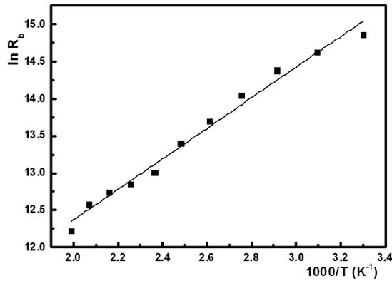
Fig. 8. Plot of  $\ln R_b$  versus  $1000/T$  of Al/p-ZnGa<sub>2</sub>Se<sub>4</sub>/n-Si/Al HJD.
