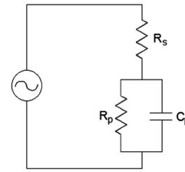
Fig. 1. Equivalent-circuit model for Al/ $p$ - $\text{ZnGa}_2\text{Se}_4/n$ -Si/Al HJD.
