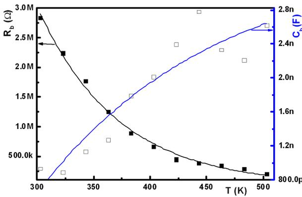
Fig. 7. Temperature dependence of the bulk resistance and capacitance of Al/p-ZnGa<sub>2</sub>Se<sub>4</sub>/n-Si/Al HJD.
