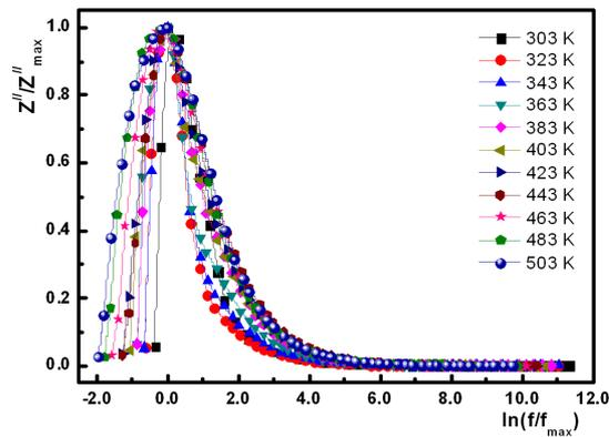
Fig. 4. Scaling behavior of  $Z''$  at various temperatures of Al/p-ZnGa<sub>2</sub>Se<sub>4</sub>/n-Si/Al HJD.
