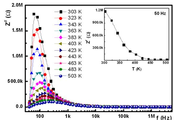
Fig. 3. Frequency dependence of the imaginary part of impedance  $Z''$  at different temperatures of Al/ $p$ - $\text{ZnGa}_2\text{Se}_4/n$ -Si/Al HJD. Inset: temperature dependence of  $Z''$  at 50 Hz.
