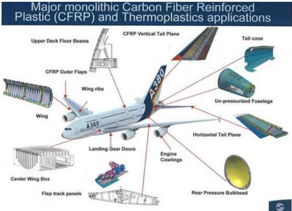
Fig. 5 Major monolithic CFRP and Thermoplastics applications [11]
