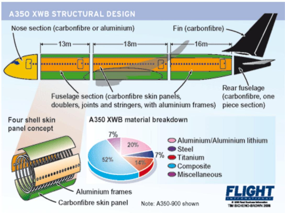
Fig. 3 Composite structure of A350XWB [22]
