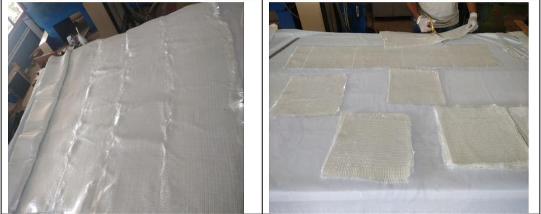
Fig. 1 - Cutting woven glass fabric in to required mould/ mold dimensions
