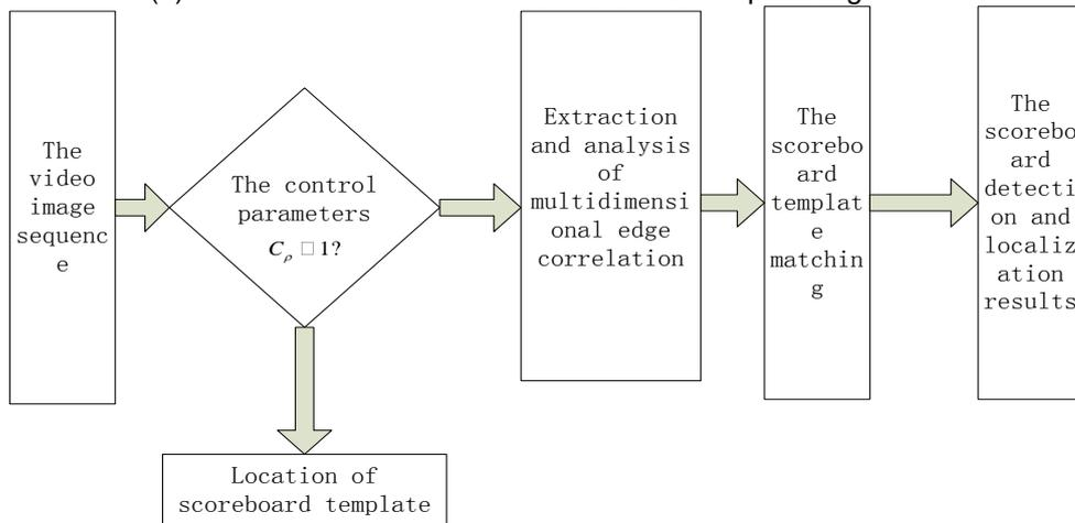
(b) The Scoreboard Monitoring Location Algorithm Based on Template Match
