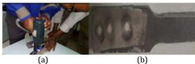
Fig. 10. (a) Chemical composition testing, (b) Spot marks after testing
