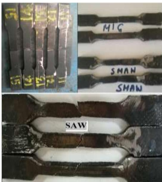
**Fig. 11.** Tensile tested non-heat treated welded specimen
