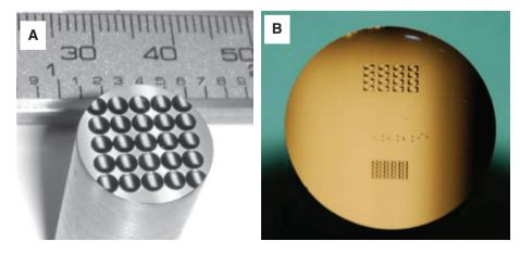
Figure 5: Freeform microlens array (A) and Alvarez lens array [19] (B) machined by SSS ultra-precision turning process [20].
