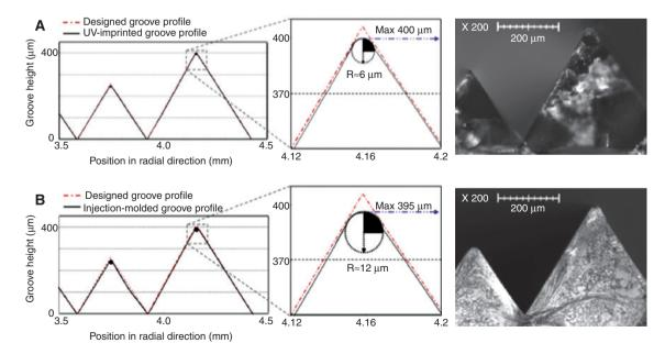
**Figure 23:** Designed and measured profile and cross-sectional images of (A) a UV-imprinted MFL with a GPR of 6 µm and (B) an injection-molded MFL with a GPR of 12 µm [63].
