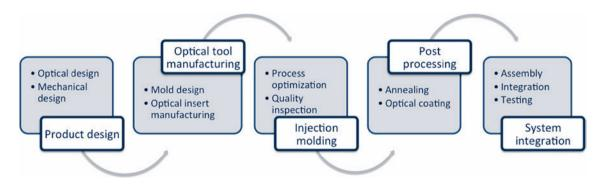
Figure 1: Process chains for manufacturing plastic optics.
