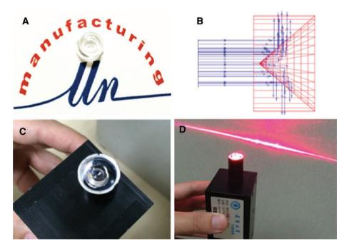
Figure 28: Laser total reflection system: (A) micro injection molded total reflection system, (B) schematic of optical path, (C) lens assembled with a laser beam, (D) laser project from sidewall of lens.
