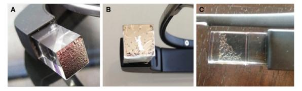
**Figure 29:** The failure of Google glasses in service: (A) bubbled surface formed on a concave reflector in a humid and hot weather [66], (B) delamination of coatings of concave reflector [67], and (C) breakage between 6-month use [68].
