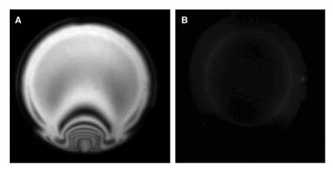
**Figure 21:** Distribution of residual birefringence: (A) preform with PV 15.31 μm, RMS 3.73 μm, (B) compression molding assisted annealing gives PV 0.693 μm and RMS 0.16 μm [60].
