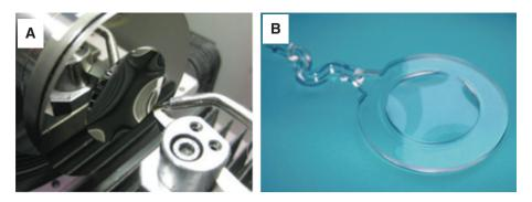
**Figure 6:** Freeform tool insert positioned at the vacuum chuck on the ultra-precision machine (A) and diamond tool and molded freeform optical element with defined Zernike surface including gate (B) [21].
