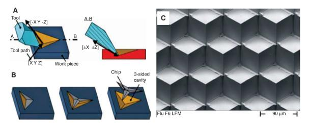
**Figure 10:** Diamond micro chiseling process for manufacturing cubic hexagon retro-reflector arrays: (A) principle of diamond micro chiseling, (B) cubic hexagon retro-reflector arrays [28], (C) the diamond micro chiseling machined cubic array with an individual circumference diameter of 100 μm on an electroless nickel substrate with intruding edges caused by interactions of set-up accuracy, non-ideal tool geometry and plastic material behavior.
