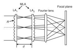
Figure 25: Structure of imaging homogenizer.
