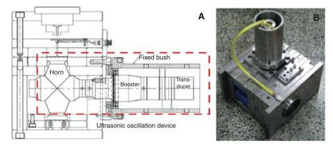
Figure 19: Ultrasonic assisted injection mold [58].
