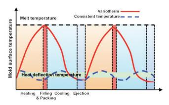
**Figure 16:** Under variotherm mold temperature control system, mold temperature increases to/over material's glass transition temperature to reduce material viscosity and flow resistance, to diminish welding lines and help surface replication. In cooling stage, mold temperature is reduced to material's deflection temperature in order to eject part out safely [49].
