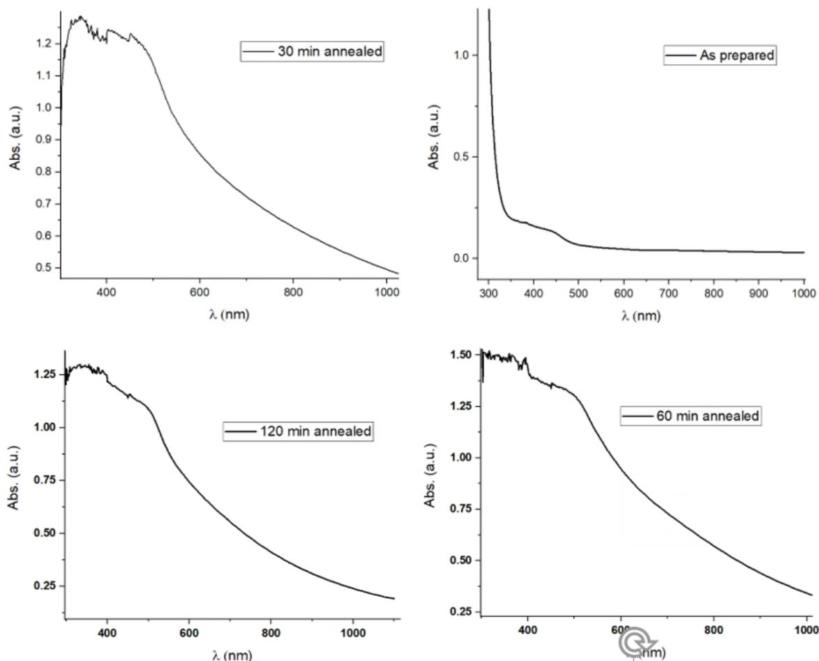
Fig. 3. UV-Visible absorption spectrums of CdZnS thin.
