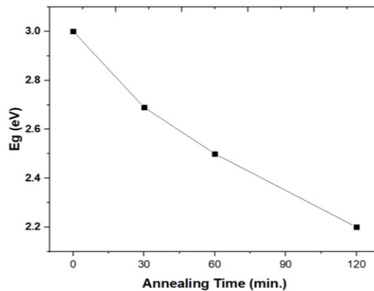
Fig. 5. Energy gap ( $E_g$ ) with annealing time for films annealed at 200 C.
