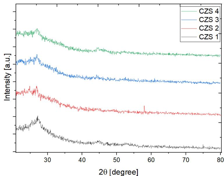
Fig. 2. X-ray diffractograms of CdZnS thin films annealed at different time CZS 1 (0 min), CZS 2 (30 min), CZS 3 (60 min), CZS 4 (120 min).
