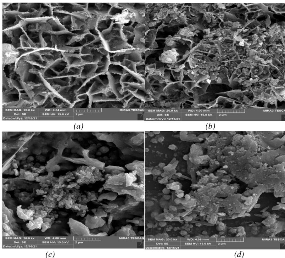
Fig. 2. FESEM images of CdZnS thin films annealed at different time
