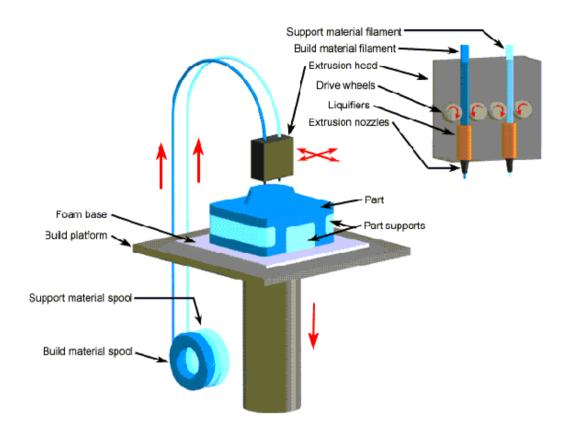
Figure 1. Schematic of FDM (Garg and Singh, 2011).
