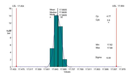
Figure 7. Histogram as per DIN standards.
