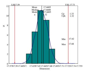
Figure 8. Histogram at reduced tolerances.
