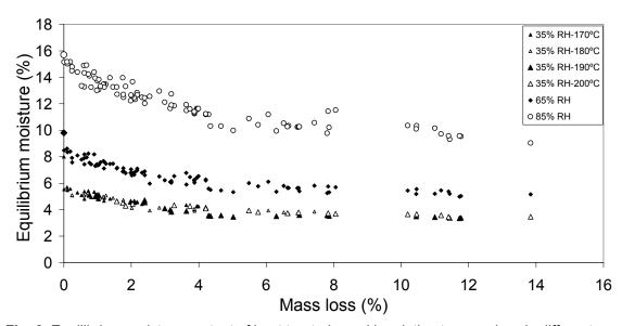
**Fig. 2.** Equilibrium moisture content of heat treated wood in relation to mass loss in different relative humidity environments.
