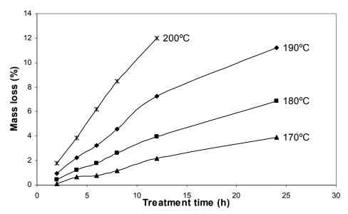
Fig. 1. Pinewood mass loss with heat treatment
