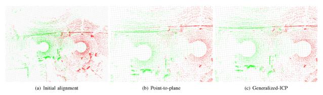
Fig. 6. Example of results for velodyne scan pair #31
