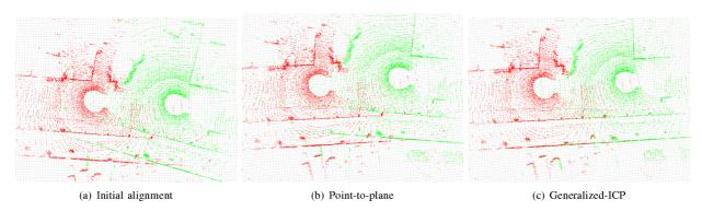
Fig. 7. Example of results for velodyne scan pair #45
