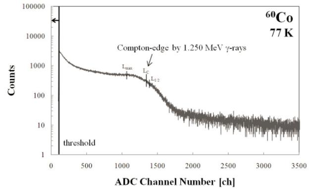
**Fig. 6** Pulse height distribution of signals in detection  $\gamma$ -rays emitted from  $^{60}\text{Co}$   $\gamma$ -ray source at 77 K.
