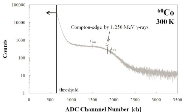
**Fig. 5** Pulse height distribution of signals in detection  $\gamma$ -rays emitted from  $^{60}\text{Co}$   $\gamma$ -ray source at 300 K.
