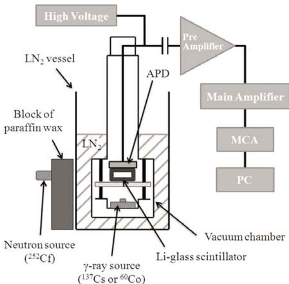
**Fig. 2** The schematic structure of experimental apparatus.
