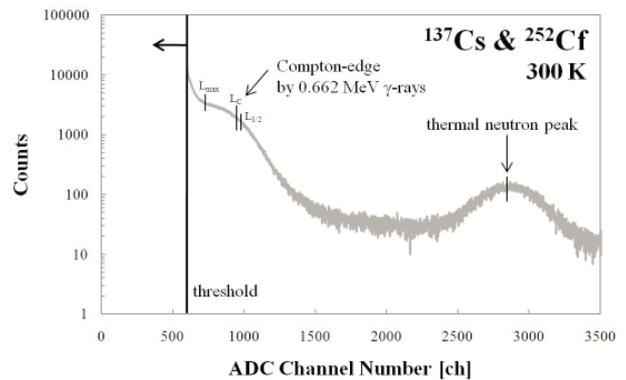
**Fig. 3** Pulse height distribution of signals in detection neutrons and  $\gamma$ -rays emitted from  $^{252}\text{Cf}$  neutron source and  $^{137}\text{Cs}$   $\gamma$ -ray source at 300 K.
