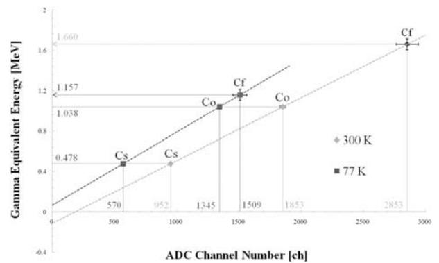
**Fig. 7** Gamma equivalent energy calibration graph.
