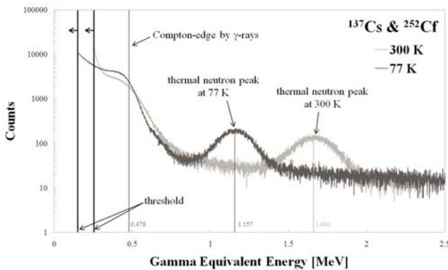
Fig. 8 Pulse height distributions concerned with gamma equivalent energy of signals in detection neutrons and  $\gamma$ -rays emitted from  $^{252}\text{Cf}$  neutron source and  $^{137}\text{Cs}$   $\gamma$ -ray source at temperature of 300 K and 77 K.
