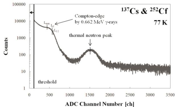
**Fig. 4** Pulse height distribution of signals in detection neutrons and  $\gamma$ -rays emitted from  $^{252}\text{Cf}$  neutron source and  $^{137}\text{Cs}$   $\gamma$ -ray source at 77 K.
