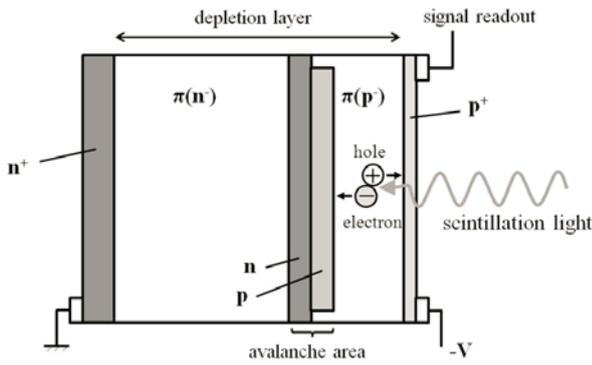
**Fig. 1** The schematic structure of avalanche photodiode (APD).
