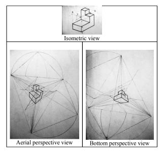
Fig. 9: Conversion of textual isometric views into perspective views through manual drafting
