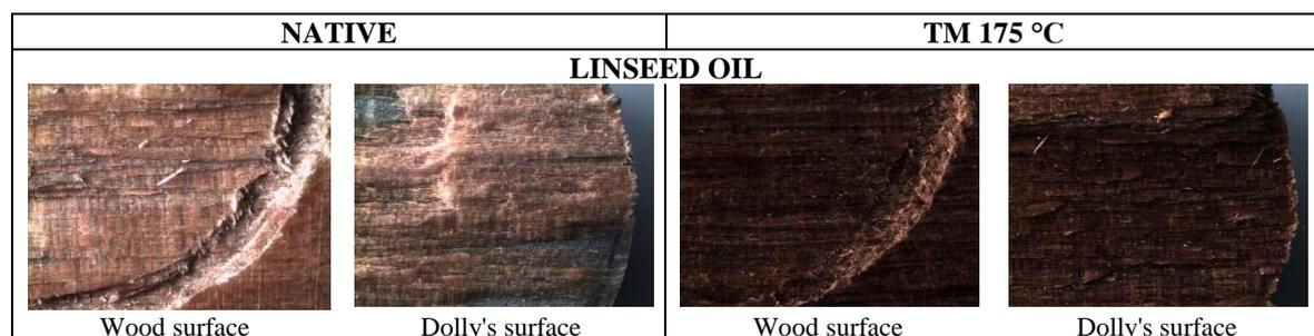
**Fig. 3 Surfaces of wood and a dolly after pulling-off the surface finish of linseed oil.**
