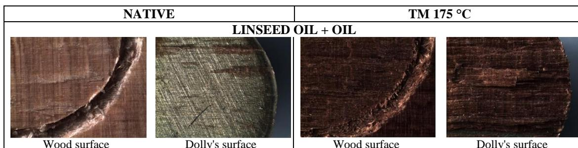
**Fig. 4 Surfaces of wood and a dolly after pull-off test of surface finish of linseed oil + oil.**
