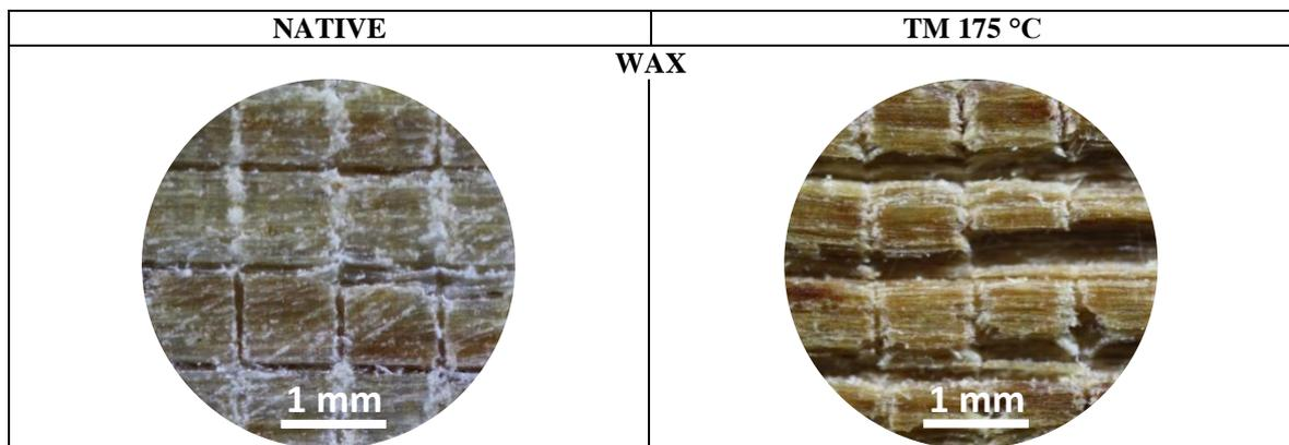
**Fig. 2 Grid damage on surface finish after Cross-cut adhesion testing.**
