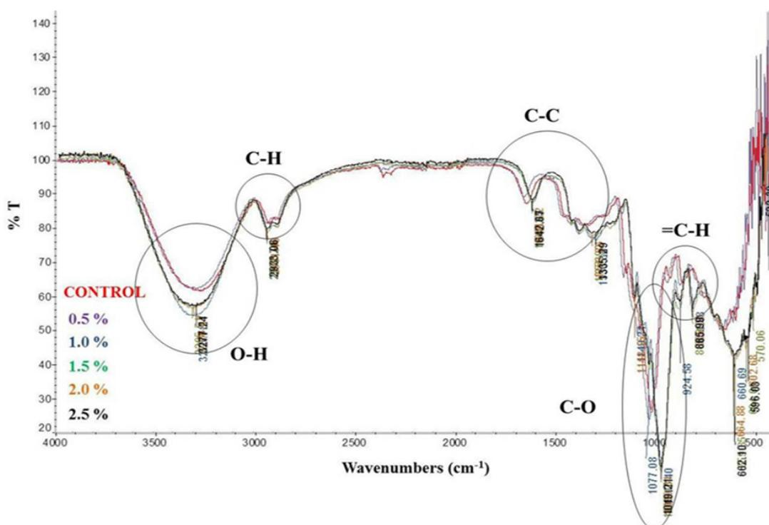
FIGURE 4. FTIR spectra of (a) Control film and (b) AM film containing thymol (0.5 - 2.5% w/v)
