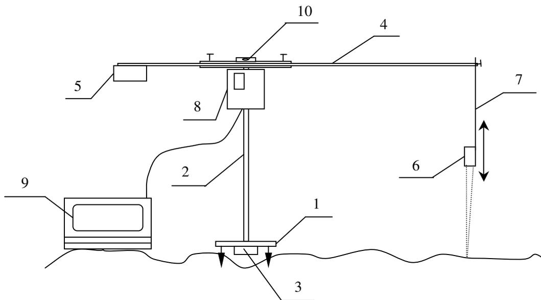
Fig. 1. Schematic diagram of profilograph design
