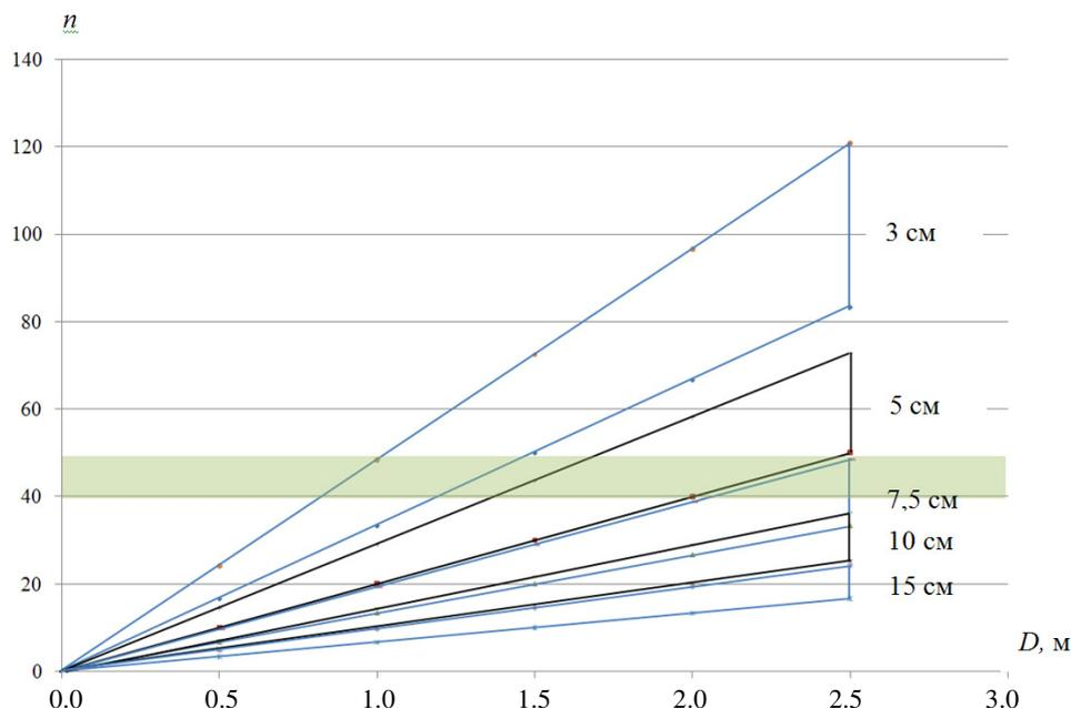
Fig. 3. Dependence of intersections number with midline on diameter of scanned circle and width of technological furrow
