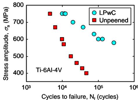
**Fig. 8** Push-pull fatigue test results of Ti-6Al-4V.
