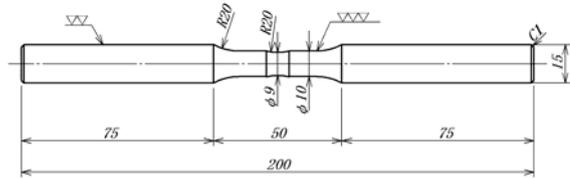
Fig. 5 Shape and dimensions of SUS316L samples.
