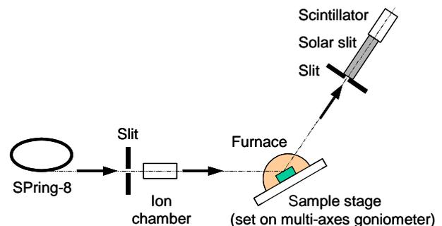
**Fig. 3** Configuration of X-ray diffraction in SPring-8.
