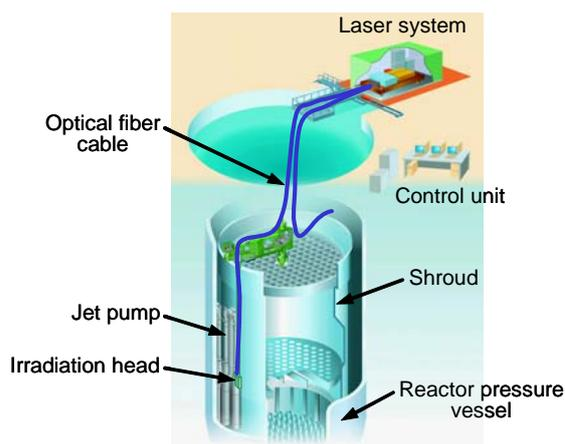
Fig. 12 LPwC system for preventive maintenance against SCC of BWR core shroud.
