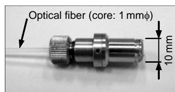
Fig. 13 Miniaturized head with optical fiber.
