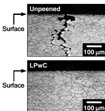
Fig. 11 SCC test results on SUS304.
