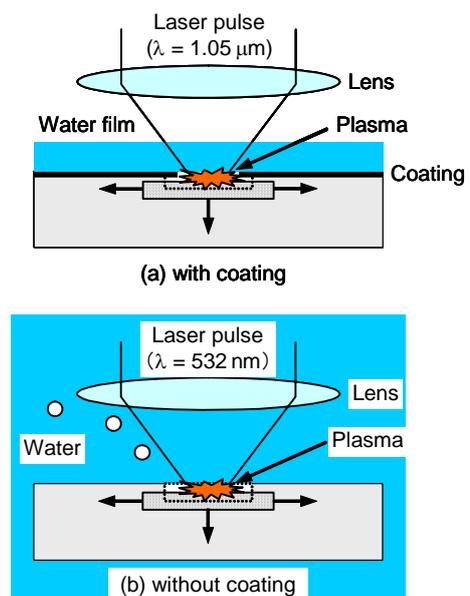
**Fig. 1** Process of laser peening.
