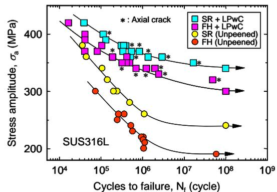
Fig. 6 Rotating-bending fatigue test results of SUS316L.
