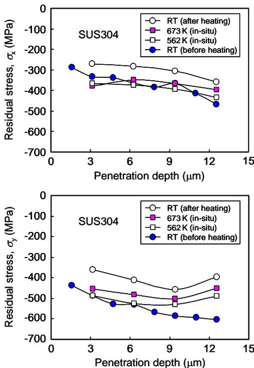
Fig. 4 Residual stress depth profile of 20 % cold-worked SUS304 processed by LPwC.
