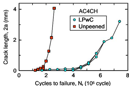
**Fig. 10** Fatigue crack propagation behavior in AC4CH.
