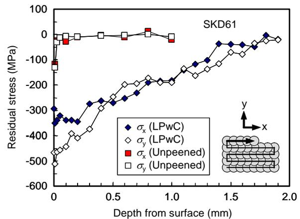
**Fig. 2** Residual stress depth profile of SKD61.
