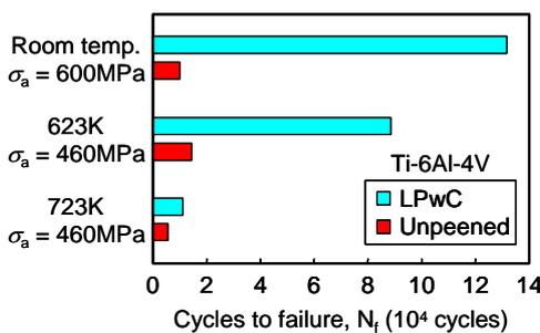
**Fig. 9** Push-pull fatigue test results of Ti-6Al-4V at elevated temperatures.
