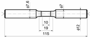
**Fig. 7** Shape and dimensions of Ti-6Al-4V samples.
