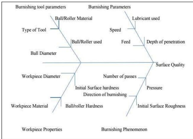
**Figure 2.** Fishbone Diagram for Burnishing Process
