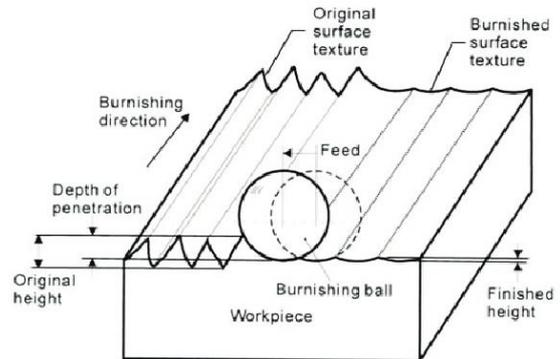
**Figure 1.** Schematic representation of burnishing operation
