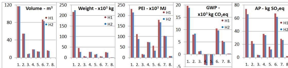
Figure 1: Environmental profile of building structures (1-underwork, 2-vertical load bearing structures, 3-partition structures, 4-ceiling, 5-roof, 6-thermal insulation, 7-surfaces, 8-doors & windows)
