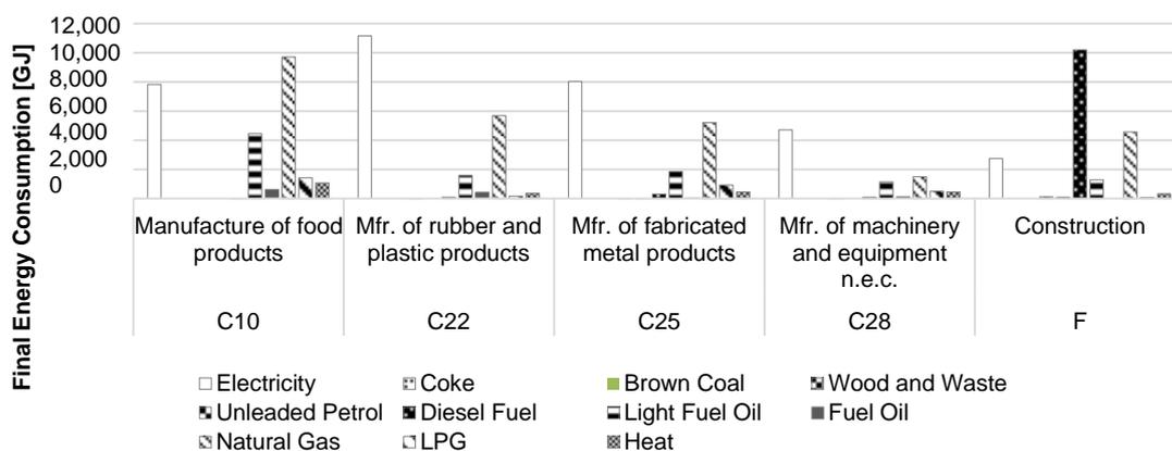
Figure 3: Energy Consumption Profile for reference medium SME for branches C10, C22, C25, C28 and F
