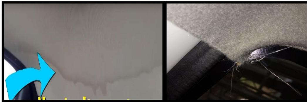
Figure 2. Defects selected for Kaizen-2 (stain marks on roof and poor cutting of mats)
