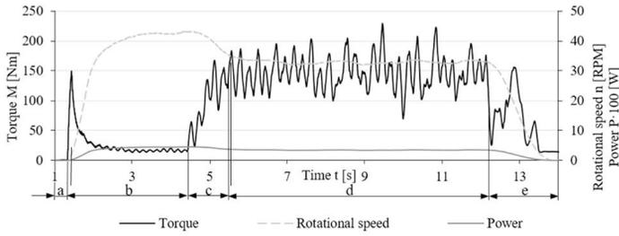
Fig. 2: Torque vs. time and RPM vs. time curves for the comminution of a laminated particle board 18 mm thick and 50 mm wide; indicated are some selected process intervals: a – machine switched off, b – mill start-up, c – comminution started, d – comminution in course, e – comminution ended.
