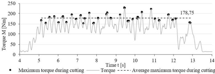
Fig. 3: Torque vs. time curve for the comminution of a laminated particle board 18 mm thick and 50 mm wide; indicated are the maximum values for the cutting process, with the determination of the arithmetic value.
