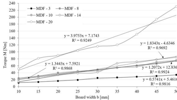
Fig. 4. Torque vs. width (of board under comminution) curves in the comminution process, taking into consideration the material and width, where at the legend of the graphs are indicated characteristics adequate for the line trend of the curves shown.
