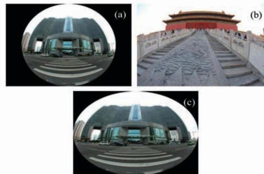
Fig. 1. Comparison of different fish-eye images. (a) Circular image generated in fish-eye lens; (b) overall fish-eye image; (c) elliptical image in anamorphic lens.
