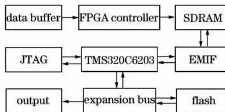
Fig. 4. Hardware configuration of the DSP system. SDRAM: synchronous dynamic random access memory; JTAG: joint test action group; EMIF: external memory interface.
