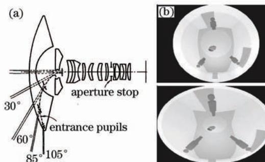
Fig. 3. Design principle of the enhanced fish-eye lens. (a) Positions of different entrance pupils; (b) two images obtained by fish-eye (upper) and enhanced fish-eye (lower) lenses. CCD surface used: 50.9% (upper), 78.5% (lower); pixels used in interesting area: 29.1% (upper), 50.3% (lower).
