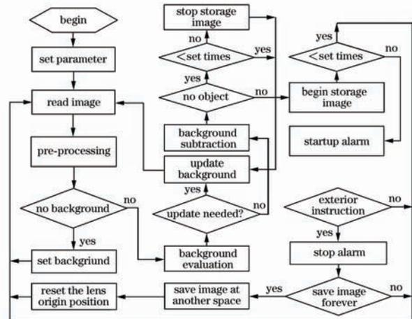
Fig. 5. DSP control and processing flow chart.
