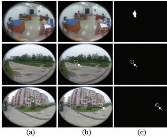
Fig. 6. Detection results of background subtraction method. (a) Background images; (b) images to be detected; (c) detection of the object.
