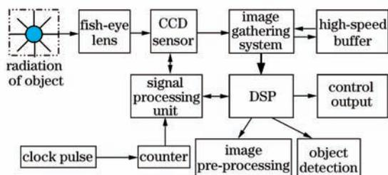
Fig. 2. Block diagram of the surveillance system.
