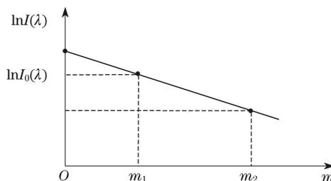
Fig. 1. Langley diagram for calibration of sun photometers.
