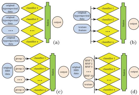
Fig. 2. Flowcharts of four feature input schemes. (a) Original data for all classifiers; (b) original data and textural feature for all classifiers; (c) different input feature sets for each classifier; (d) MNF components and texture for all classifiers.
