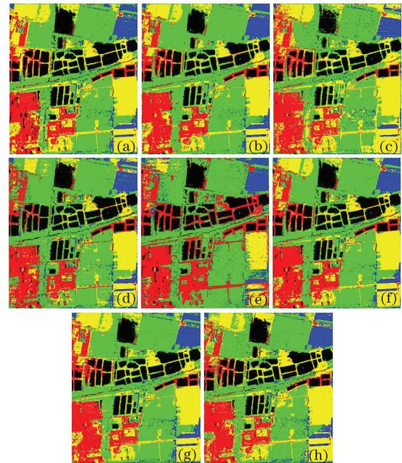
Fig. 5. Classification results of the second scheme. (a) SVM; (b) BPNN; (c) DTC; (d) MDC; (e) MLC; (f) evidence theory; (g) linear consensus; (h) SVM combiner.
