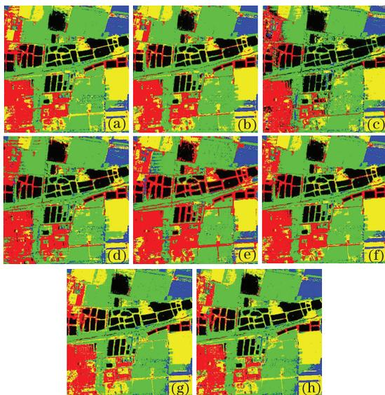
Fig. 7. Classification results of the fourth scheme. (a) SVM; (b) BPNN; (c) DTC; (d) MDC; (e) MLC; (f) evidence theory; (g) linear consensus; (h) SVM combiner.
