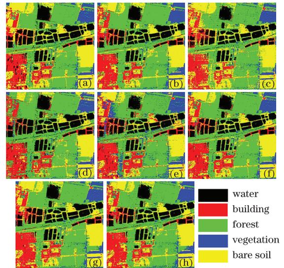
Fig. 4. Classification results of the first scheme. (a) SVM; (b) BPNN; (c) DTC; (d) MDC; (e) MLC; (f) evidence theory; (g) linear consensus; (h) SVM combiner.
