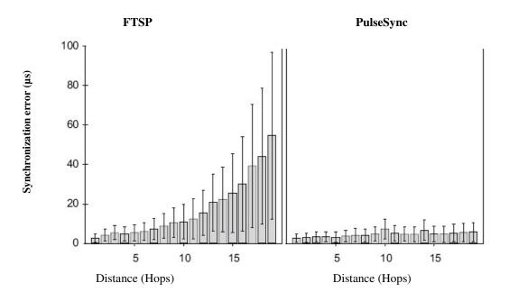
Figure 3: Synchronization error in (µS) vs number of Hops for FTSP and PulseSync
