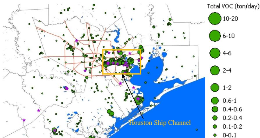
**Fig. 1.** Map centered on the Houston metropolitan area, showing highways (red lines) and  $\text{NO}_x$  and VOC point sources.  $\text{NO}_x$  point sources from Continuous Emission Monitoring System (CEMS) are shown by purple stars. Green circles indicate total VOC emissions rate (tons/day) from point sources during TexAQS 2006 (data source: Texas Commission on Environmental Quality). The Houston Ship Channel is identified by a yellow frame.
