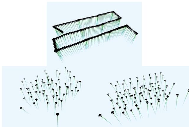
Figure 3: Camera stations for Scenario 1 (above), 2 and 3 (below)
