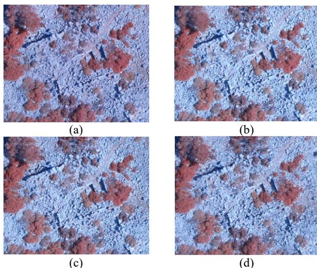
Figure 7: Orthophotos produced by Agisoft (a), Pix4D (b), Agisoft+SURE (c), Pix4D+SURE (d) for Scenario 3
