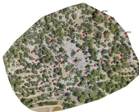
Figure 2: Area of interest and distribution of the Ground Control Points
