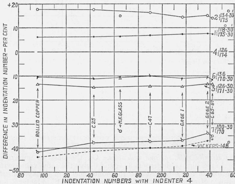
FIGURE 9.—Indentation numbers based on penetration ( $I = \sqrt{\text{load}/\text{penetration}}$ ).
