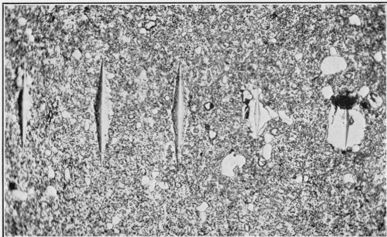
FIGURE 15.—*Indentations in a molybdenum-tungsten-cobalt steel containing large carbide particles (magnification,  $\times 500$ ).*
