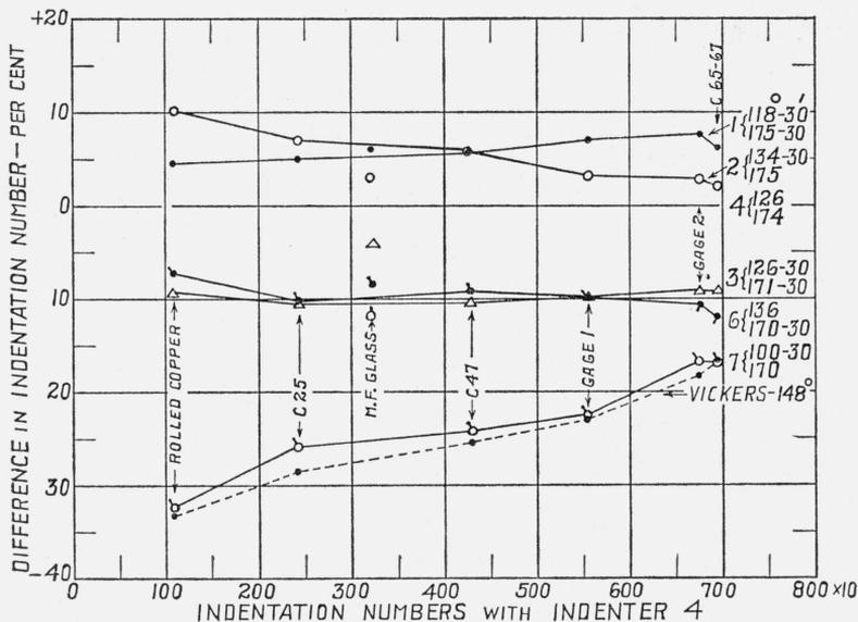
FIGURE 10.—Indentation numbers based on volume ( $I = \text{load}/(\text{volume})^{2/3}$ ).
