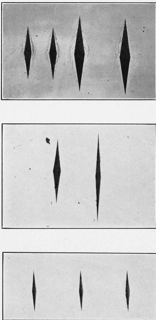
FIGURE 6.—*Indentations in specimens having different elasticities.*
