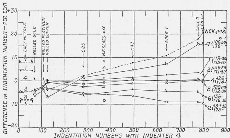
FIGURE 12.—Indentation numbers based on unrecovered projected area.
