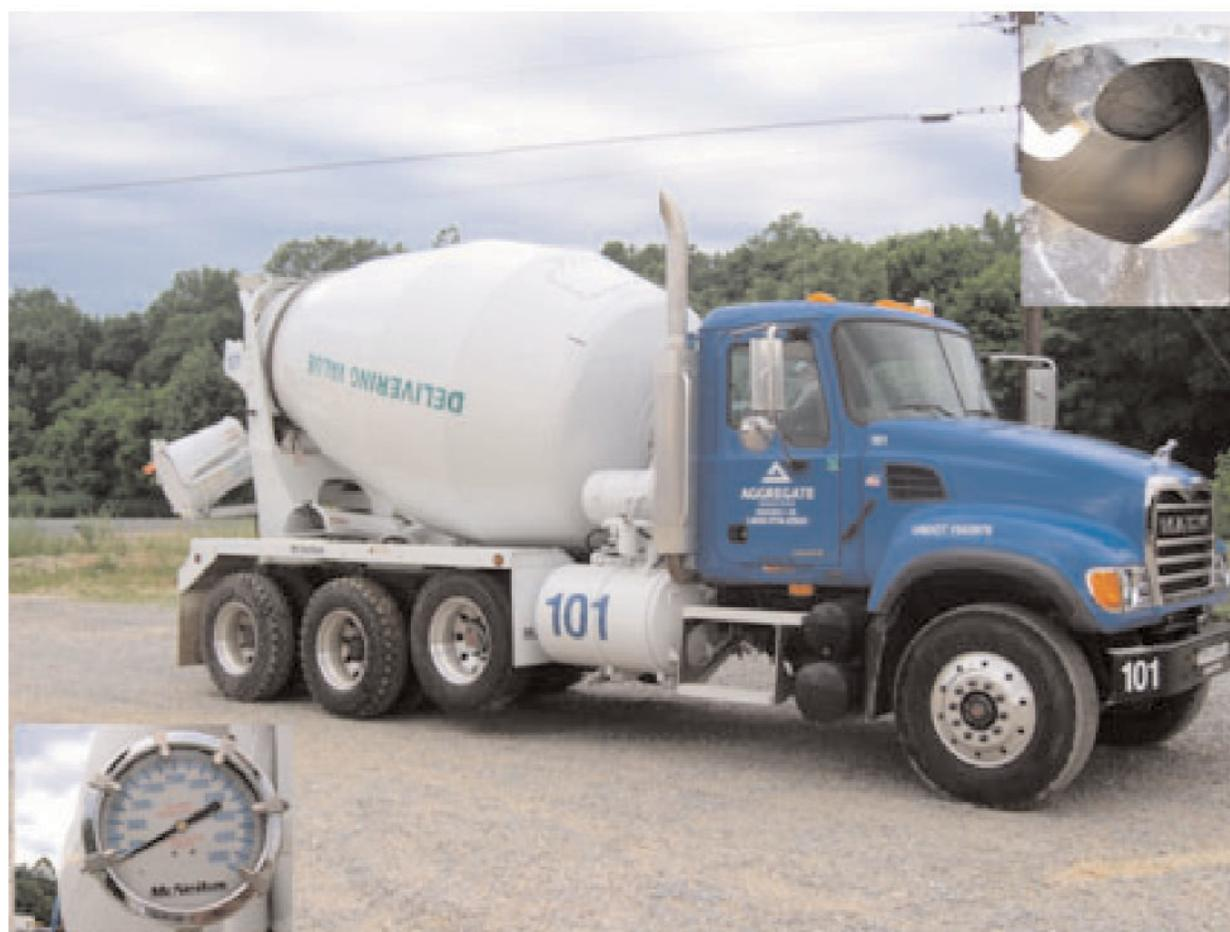
**Fig. 1.** View of the used truck, the slump indicator (bottom left) and the interior of the drum (top right).
