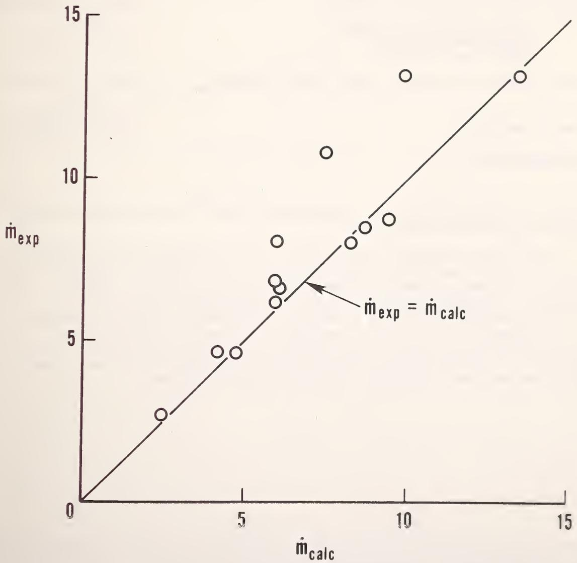
Figure 17. Calculated mass flow rate vs experimental mass flow rate
