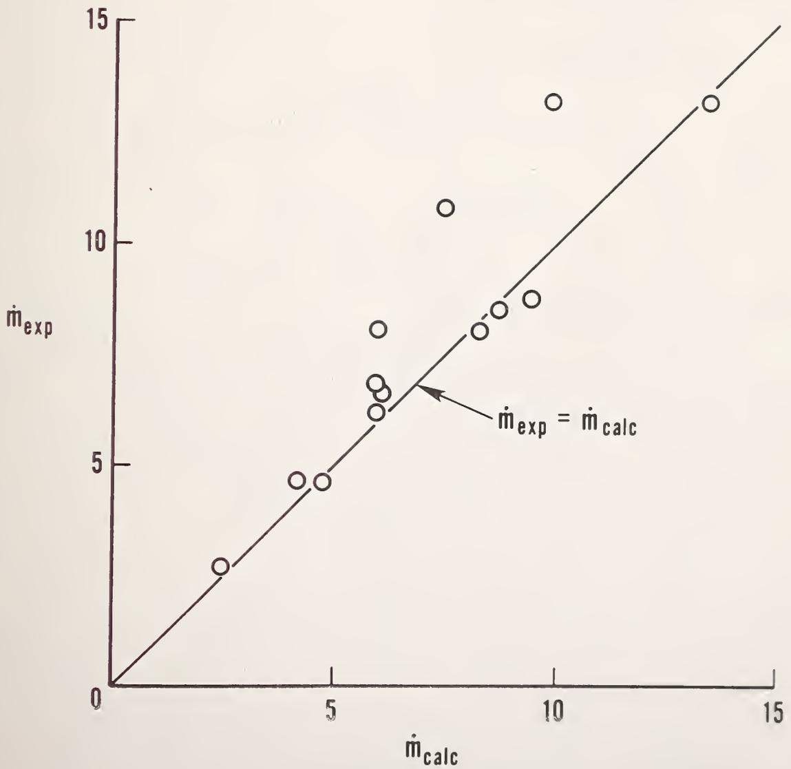
Figure 17. Calculated mass flow rate vs experimental mass flow rate
