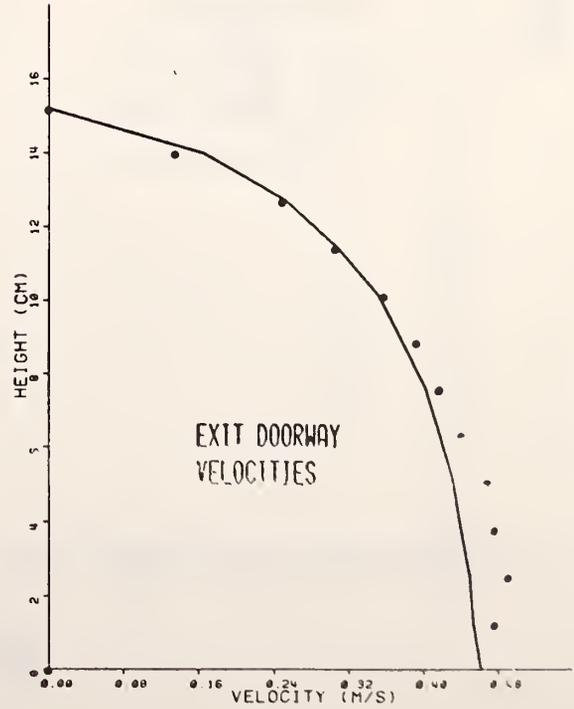
Figure 14. Experimental temperature and velocity results and calculated velocities for  $W_E/W_D = 0.6$
