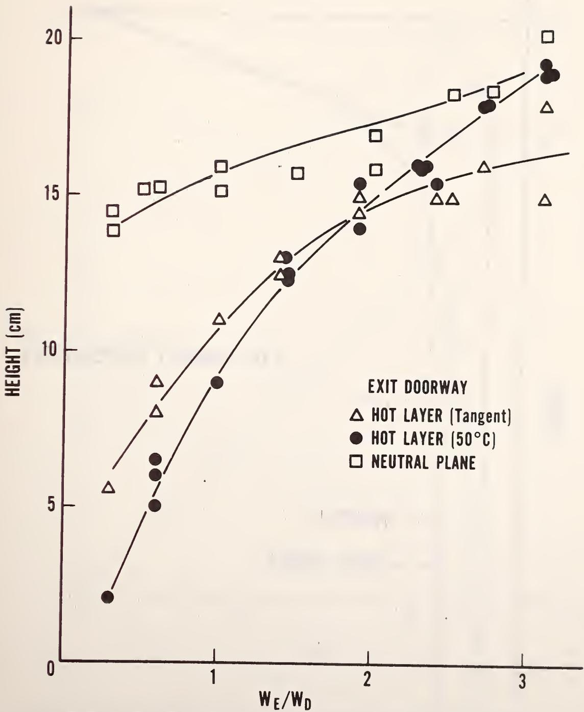
Figure 15b. Neutral plane height and effective height of hot layer based on corridor temperature adjacent to exit doorway vs  $W_E/W_D$
