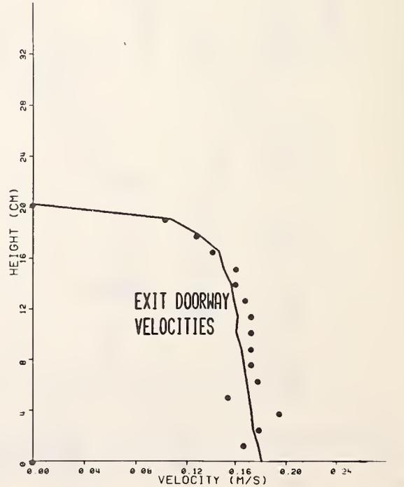
Figure 11. Experimental temperature and velocity results and calculated velocities for  $W_E/W_D = 3.1$
