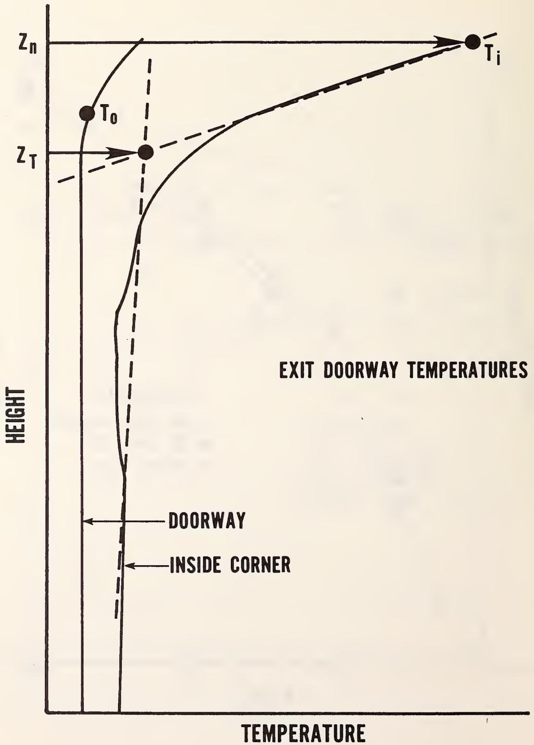
Figure 16. Example of determination of  $z_T$ ,  $z_n$ ,  $T_i$  and  $T_o$  from temperature data
