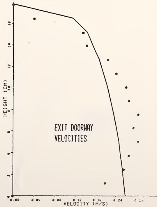
Figure 12. Experimental temperature and velocity results and calculated velocities for  $W_E/W_D = 1.9$
