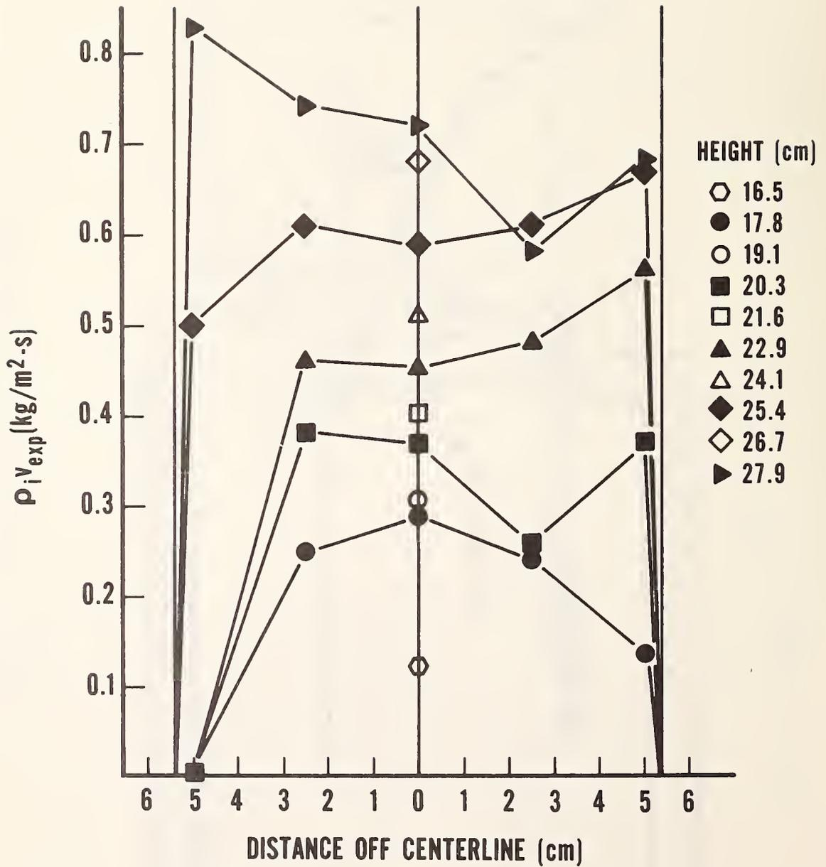
Figure 7. Mass flow rates for flow out the exit doorway
