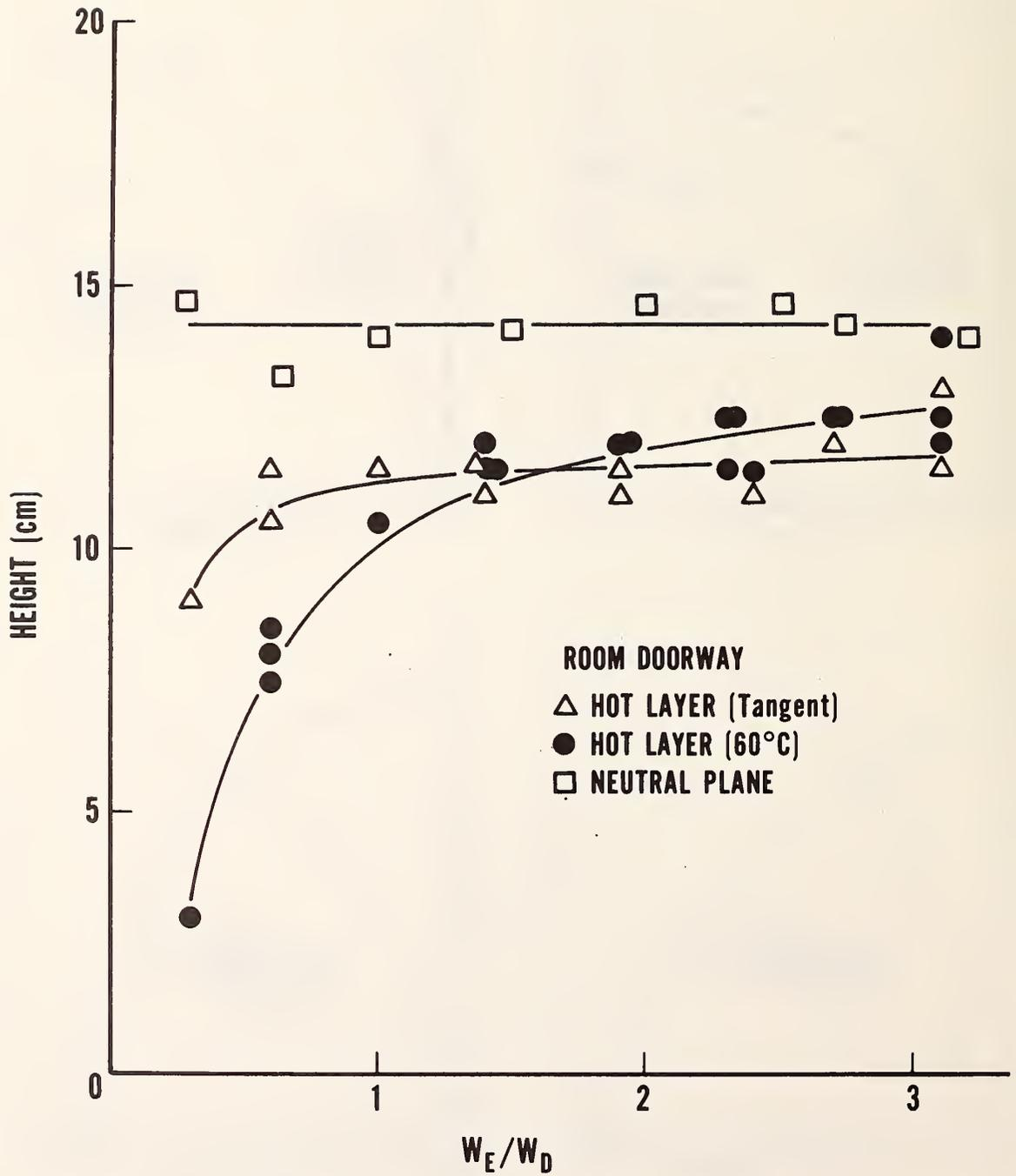
Figure 15a. Neutral plane height and effective height of hot layer based on room doorway temperature vs  $W_E/W_D$
