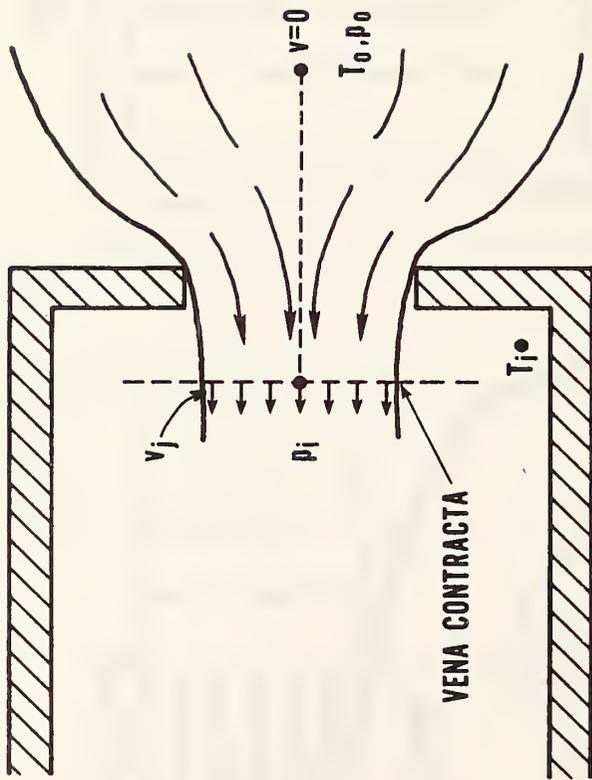
Figure 5. Diagram of vena contracta for inflow (horizontal section)
