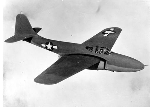
*The first GE jet engine powered Bell's experimental XP-59 aircraft.*
