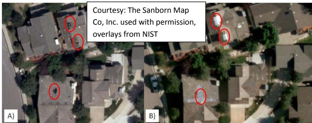
**Figure 7 Post-fire aerial images of damaged wood roofs. A). Aerial image recorded on 6/28/2012 showing black marks on wood shake roofs. B). Aerial image recorded on 7/12/2012 showing initial repairs to roofs.**
