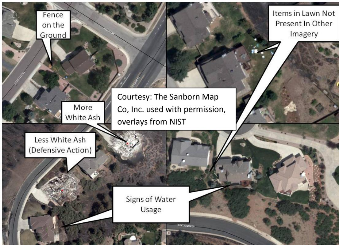
**Figure 9** Examples of remote sensing identified defensive action signs not identified during the TD process.
