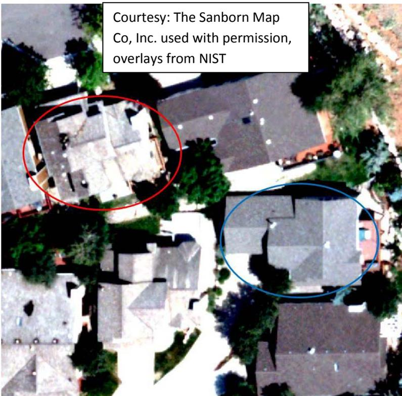
**Figure 8** Two potentially fire damaged roofs. The primary structure circled in blue had anecdotal accounts of damage from the homeowner while the structure in red has clear visible evidence of damage.
