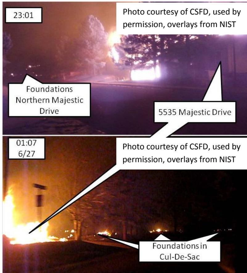
**Figure 45 Ignitions on Majestic Drive providing evidence for majority of primary structures on east side ignited or destroyed by 23:00.**
