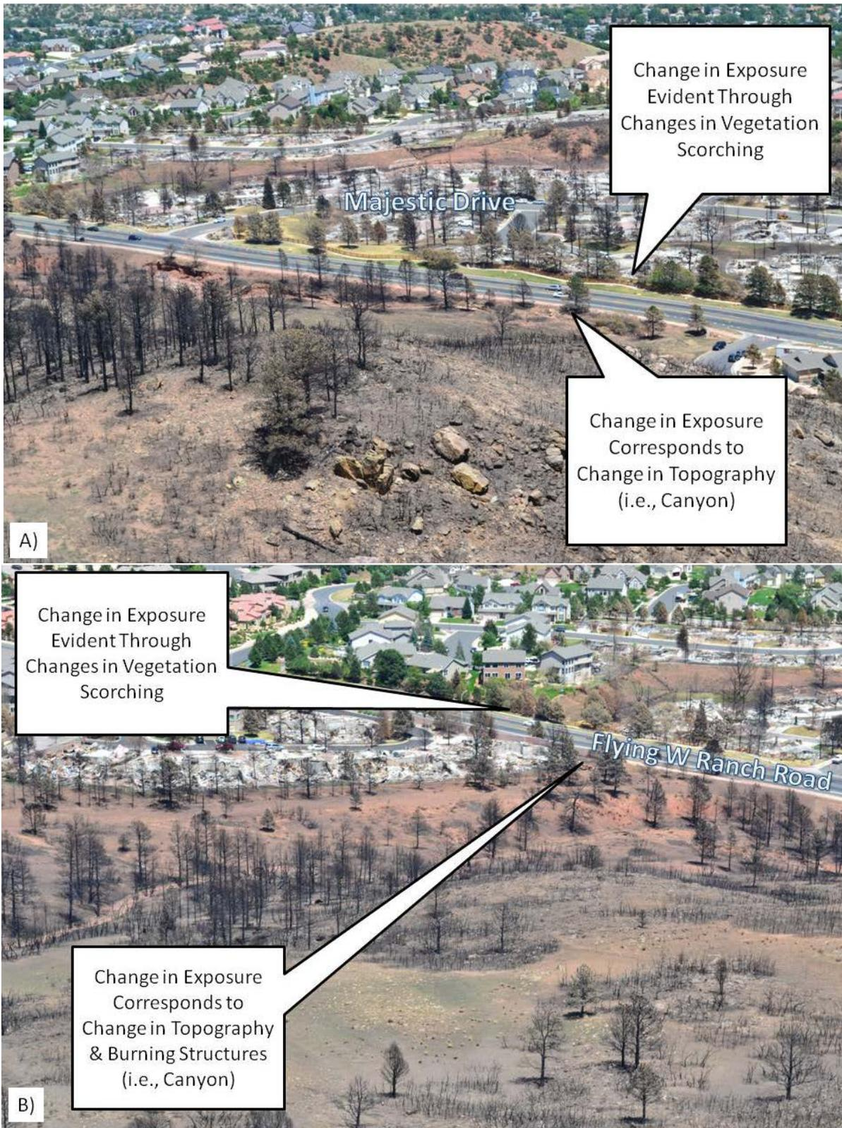
**Figure 57** Changes in exposure conditions evident through changes in scorching to vegetation corresponding to areas across from a canyon and burning structures. Looking east to northeast. NIST Photos
