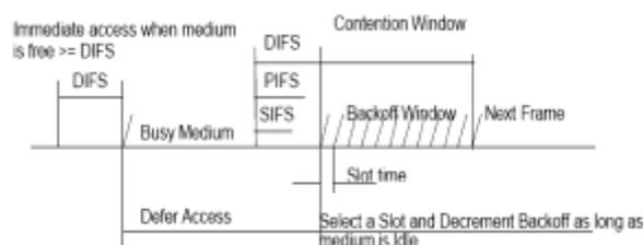
Fig 1: The Timing Relationship of DCF [7]
