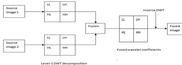
Figure-2. DWT based image fusion
