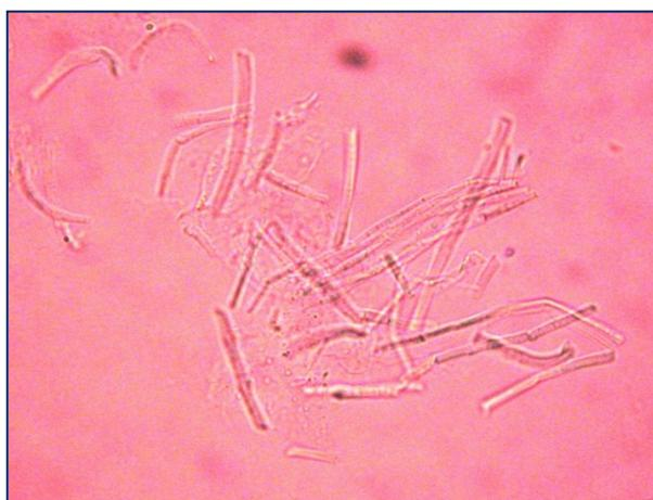
Figure 1 Microscope image for coconut coir fiber after mechanical treatment (ball milling)
