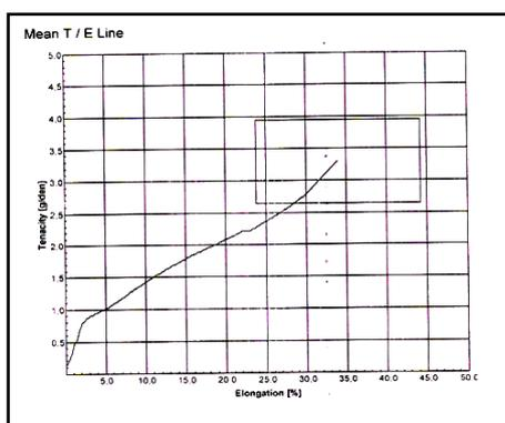
Fig. 8: Mean Tenacity vs E Line Graph of Undyed Corn Fiber
