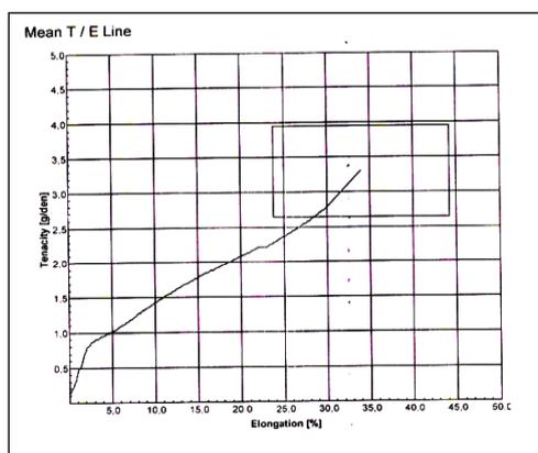
Fig. 9: Mean Tenacity vs E Line Graph of Dyed Corn Fiber at 90<sup>o</sup>C
