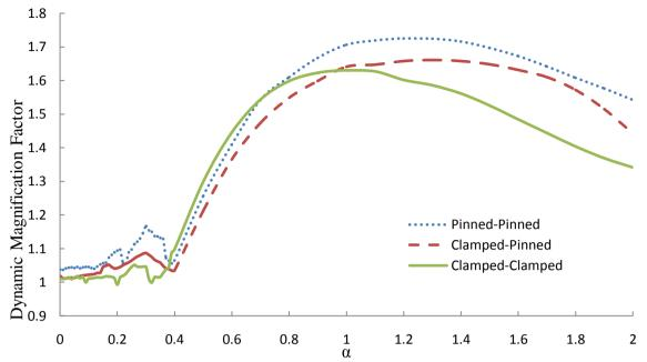
Figu10 dynamic magnification factor of the mid - point of the beam versus α for three different boundary conditions.
