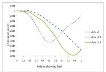
Fig 7 Dynamic displacements of the mid – point of the clamped – pinned beam versus the position of the Moving load on the beam for various α values
