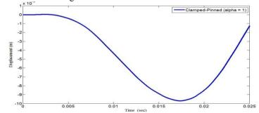
Fig 6 Matlab results for clamped –pinned boundary conditions of a beam with  $\Box \Box \Box \Box$  value
