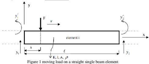
In beam structures, the beams are joined together by welding (not by pins or hinges, as in the case of truss elements), so that both forces and moments can be transmitted between the beams. The cross-section of the beam structure is assumed uniform. If a beam has a varying cross-section, it is advised that the beam should be
