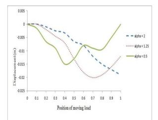
Fig 9 Dynamic displacements of the mid – point of the pinned – pinned beam versus the position of the moving load on the beam for various α values
