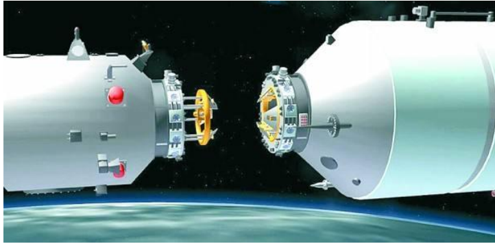
Space Rendezvous and Docking (SRD) between Shenzhou and Tiangong
