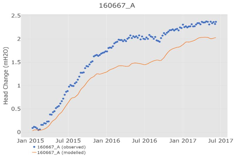
Figure S17 Modelled and observed change in groundwater level at well 160667\_A
