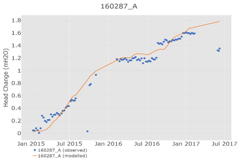
Figure S6 Modelled and observed change in groundwater level at well 160287\_A
