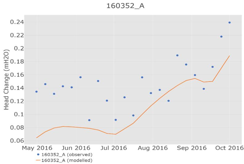
Figure S8 Modelled and observed change in groundwater level at well 160352\_A
