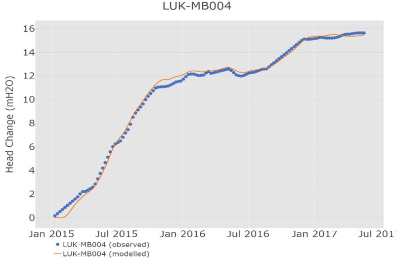
Figure S39 Modelled and observed change in groundwater level at well LUK-MB004
