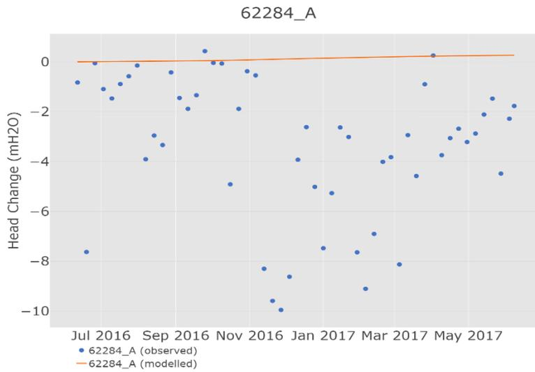
Figure S29 Modelled and observed change in groundwater level at well 62284\_A
