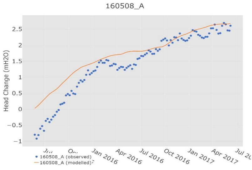
Figure S12 Modelled and observed change in groundwater level at well 160508\_A
