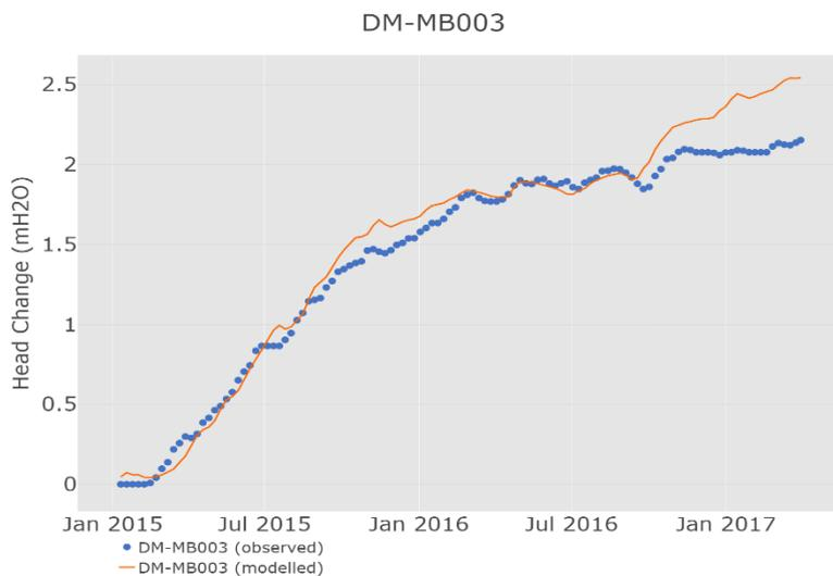
Figure S36 Modelled and observed change in groundwater level at well DM-MB003
