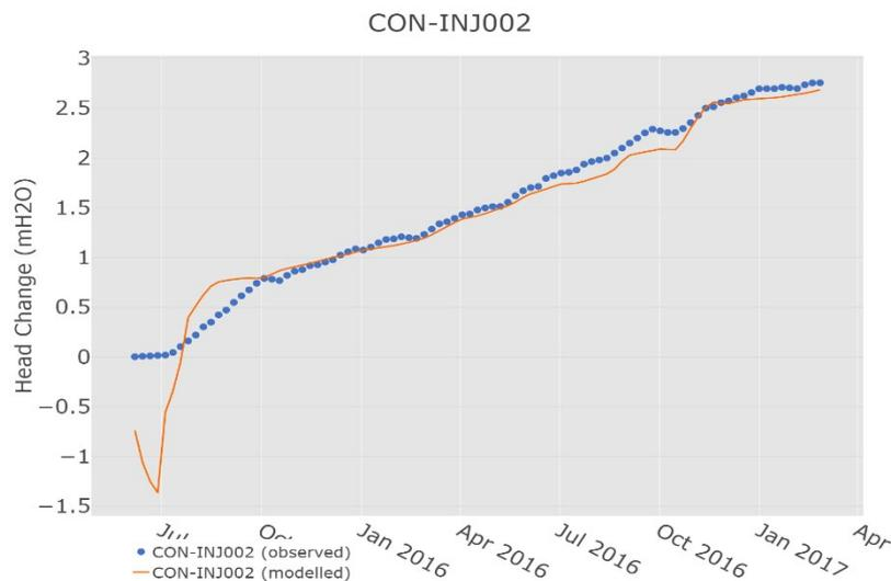
Figure S33 Modelled and observed change in groundwater level at well CON-INJ002
