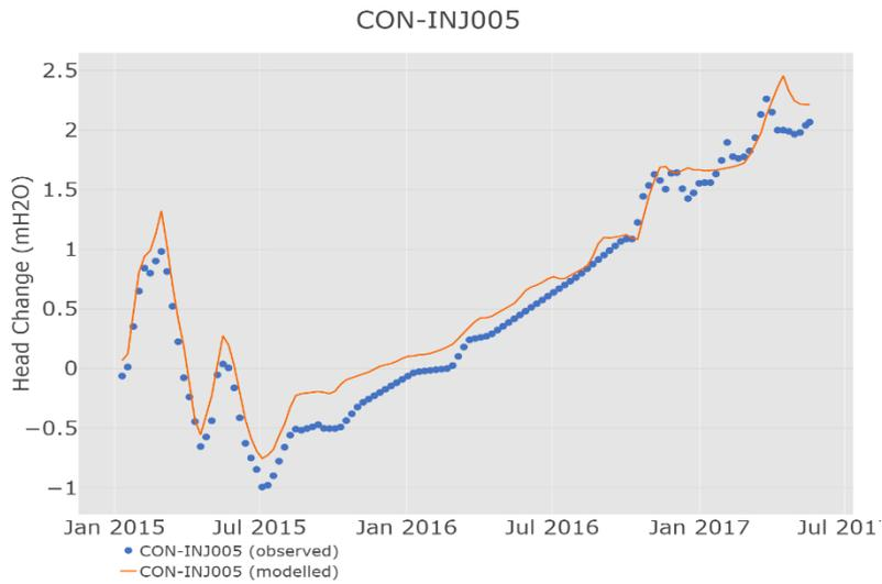
Figure S34 Modelled and observed change in groundwater level at well CON-INJ005
