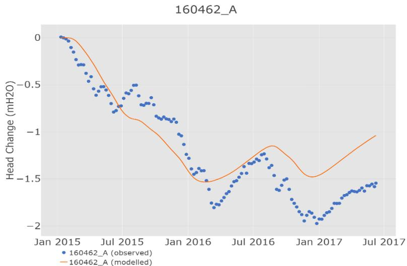
Figure S9 Modelled and observed change in groundwater level at well 160462\_A
