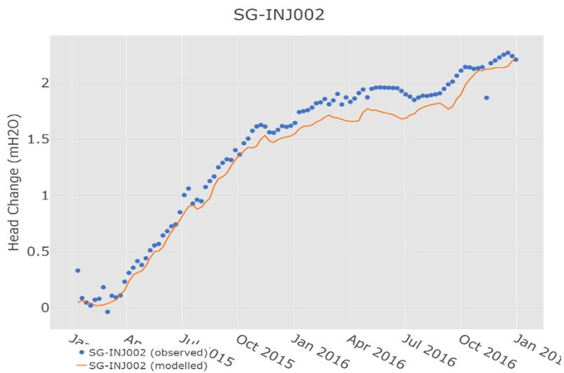
Figure S42 Modelled and observed change in groundwater level at well SG-INJ002
