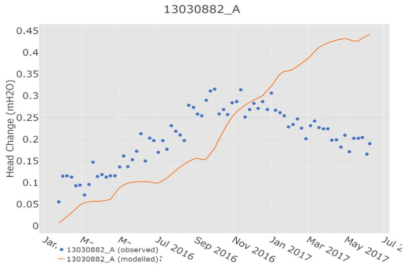
Figure S5 Modelled and observed change in groundwater level at well 13030882\_A
