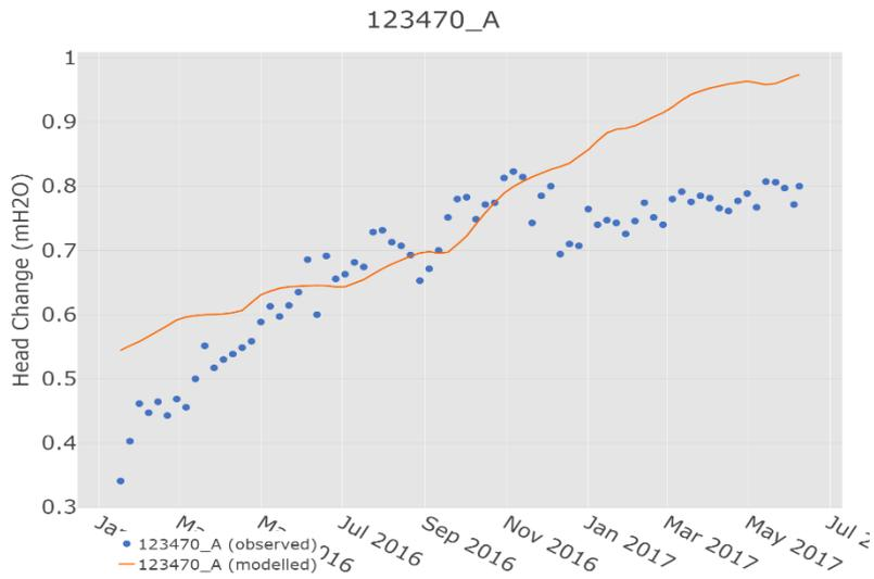
Figure S4 Modelled and observed change in groundwater level at well 123470\_A
