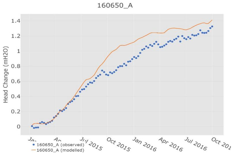
Figure S14 Modelled and observed change in groundwater level at well 160650\_A
