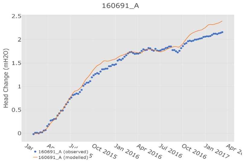
Figure S20 Modelled and observed change in groundwater level at well 160691\_A
