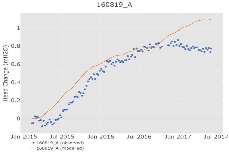
Figure S25 Modelled and observed change in groundwater level at well 160819\_A
