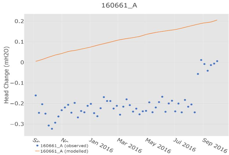
Figure S16 Modelled and observed change in groundwater level at well 160661\_A
