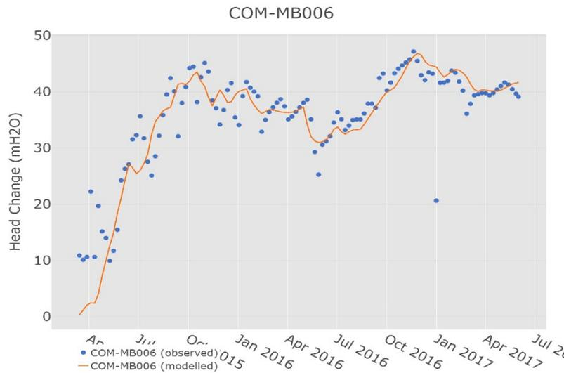
Figure S32 Modelled and observed change in groundwater level at well COM-MB006
