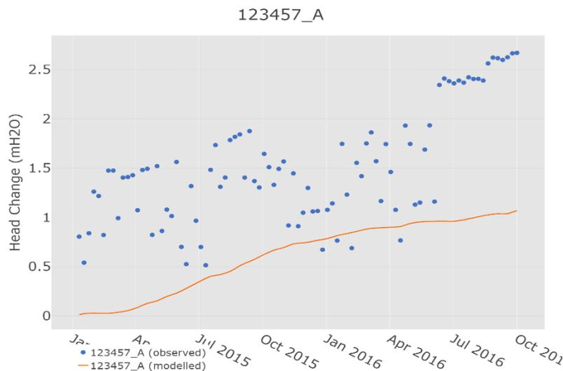
Figure S3 Modelled and observed change in groundwater level at well 123457\_A
