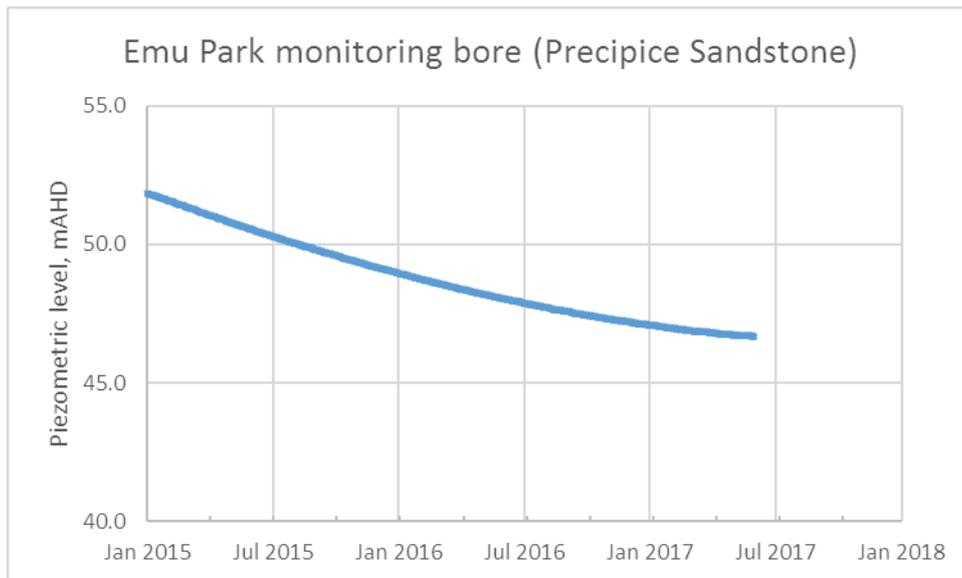
Figure S46 Observed change in groundwater level at the Emu Park bore demonstrating no response to MAR injection
