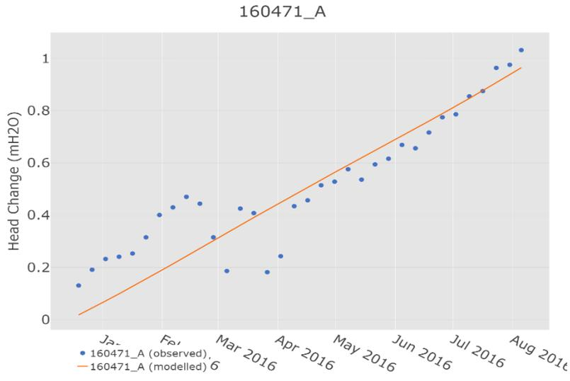
Figure S10 Modelled and observed change in groundwater level at well 160471\_A
