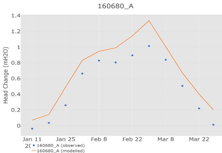
Figure S18 Modelled and observed change in groundwater level at well 160680\_A
