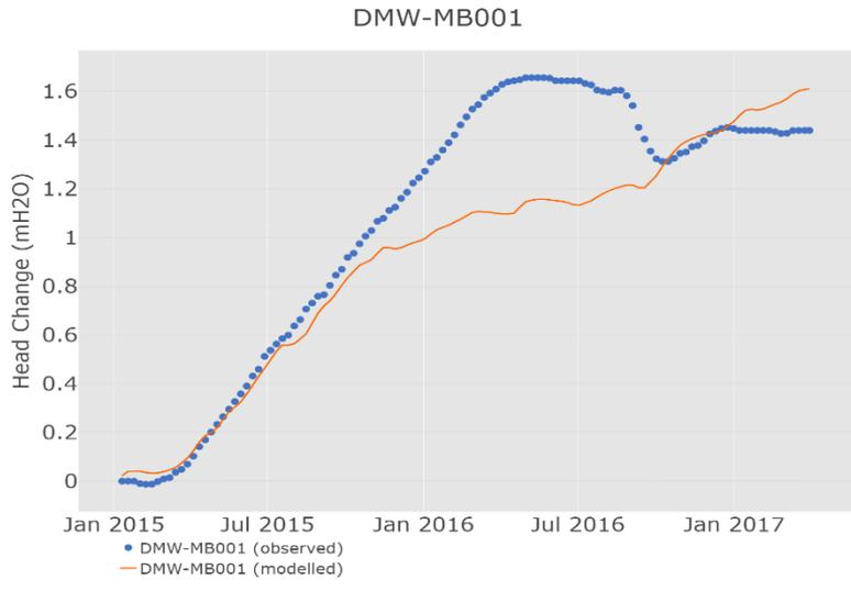
Figure S37 Modelled and observed change in groundwater level at well DMW-MB001
