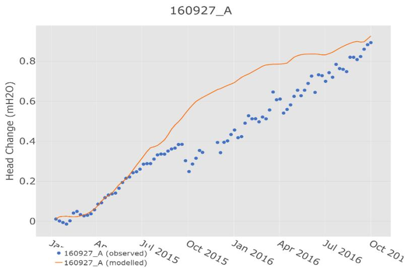
Figure S27 Modelled and observed change in groundwater level at well 160927\_A
