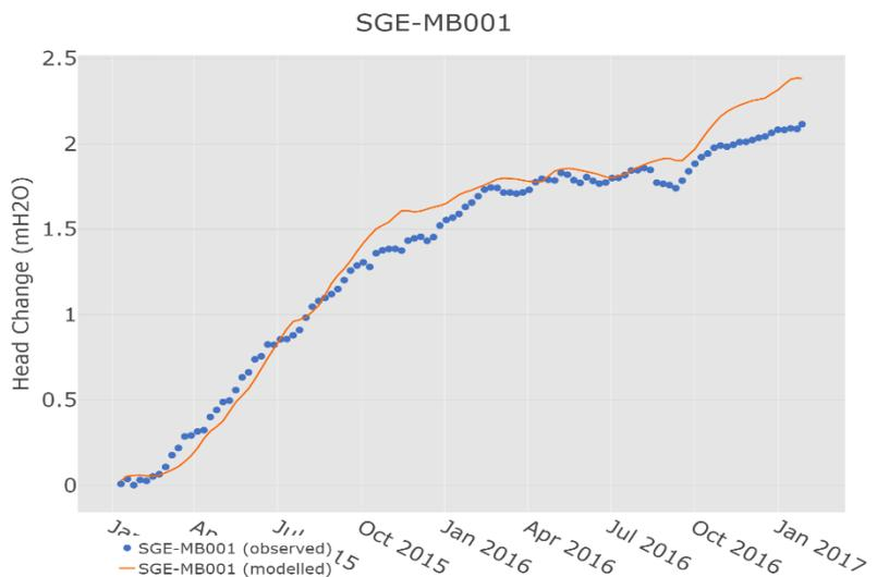
Figure S45 Modelled and observed change in groundwater level at well SGE-MB001
