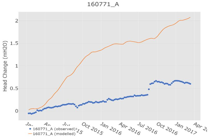
Figure S22 Modelled and observed change in groundwater level at well 160771\_A
