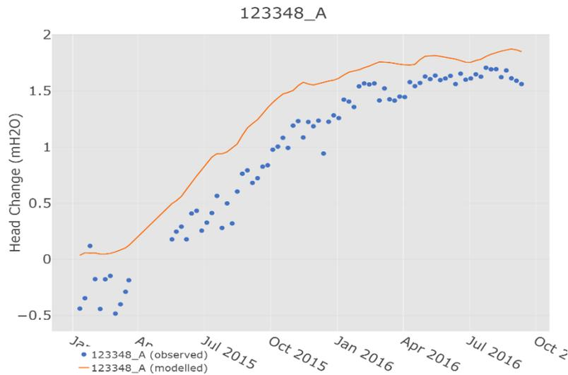
Figure S2 Modelled and observed change in groundwater level at well 123348\_A
