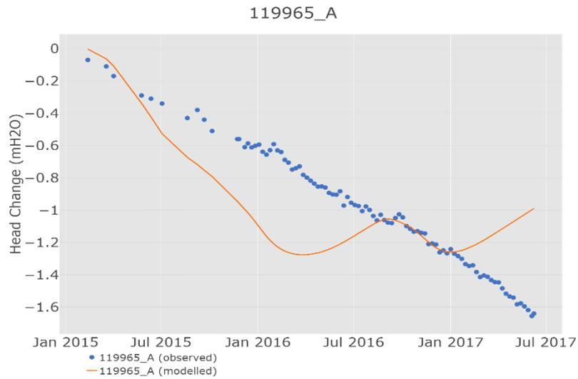
Figure S1 Modelled and observed change in groundwater level at well 119965\_A
