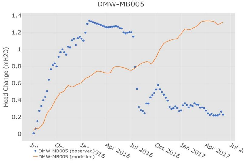
Figure S38 Modelled and observed change in groundwater level at well DMW-MB005
