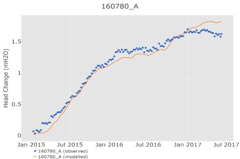
Figure S24 Modelled and observed change in groundwater level at well 160780\_A
