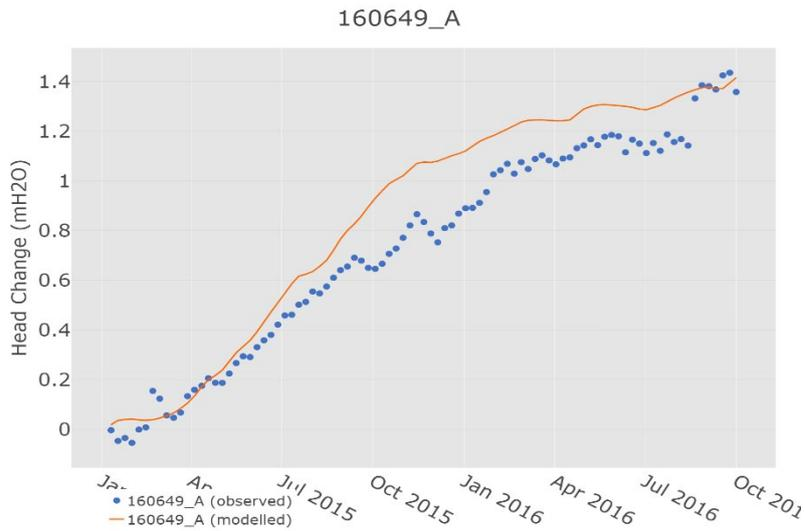
Figure S13 Modelled and observed change in groundwater level at well 160649\_A
