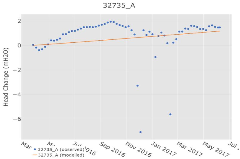
Figure S28 Modelled and observed change in groundwater level at well 32735\_A
