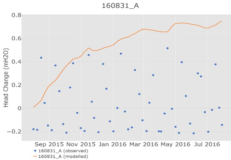
Figure S26 Modelled and observed change in groundwater level at well 160831\_A
