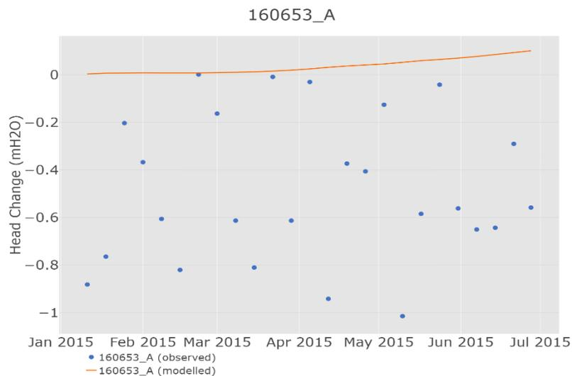
Figure S15 Modelled and observed change in groundwater level at well 160653\_A
