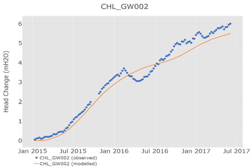
Figure S30 Modelled and observed change in groundwater level at well CHL\_GW002
