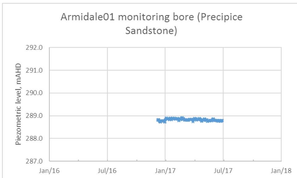
Figure S47 Observed change in groundwater level at the Armidale01 bore demonstrating no response to MAR injection
