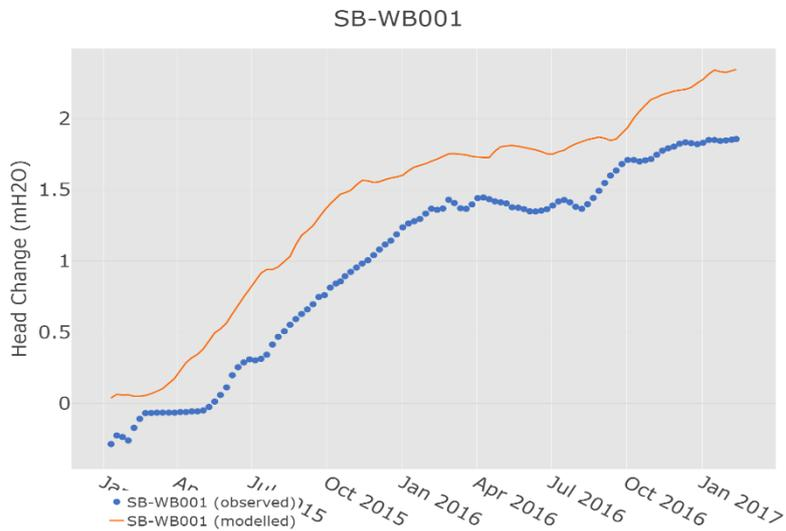
Figure S41 Modelled and observed change in groundwater level at well SB-WB001
