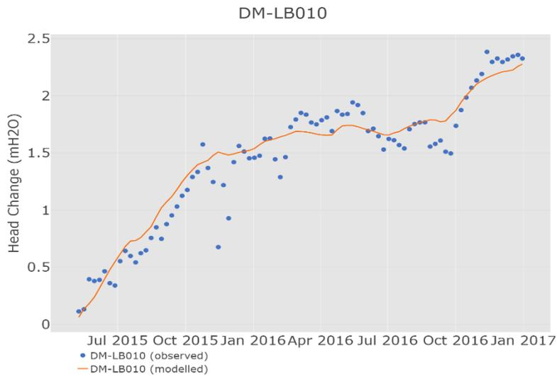
Figure S35 Modelled and observed change in groundwater level at well DM-LB010
