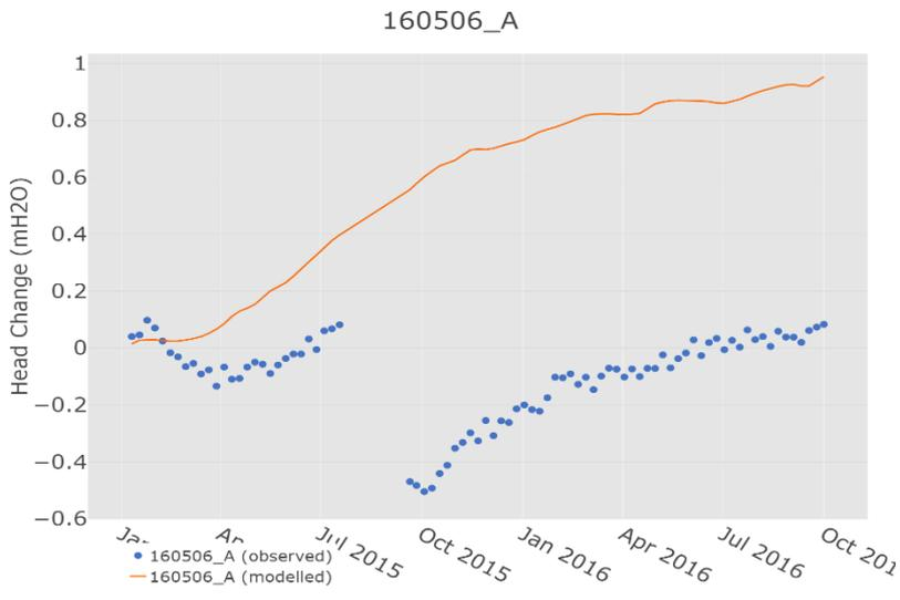
Figure S11 Modelled and observed change in groundwater level at well 160506\_A
