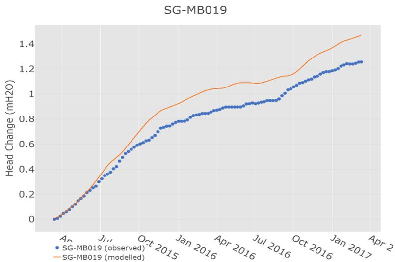
Figure S44 Modelled and observed change in groundwater level at well SG-MB019
