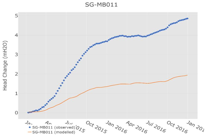
Figure S43 Modelled and observed change in groundwater level at well SG-MB011
