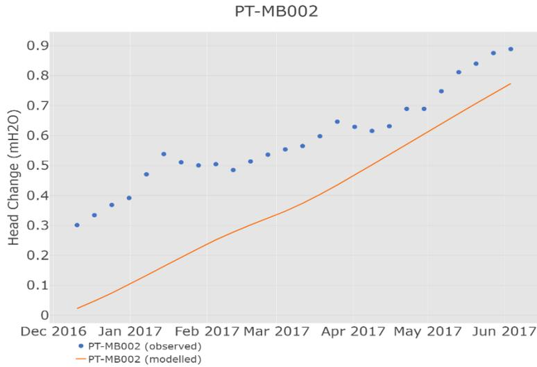
Figure S40 Modelled and observed change in groundwater level at well PT-MB002
