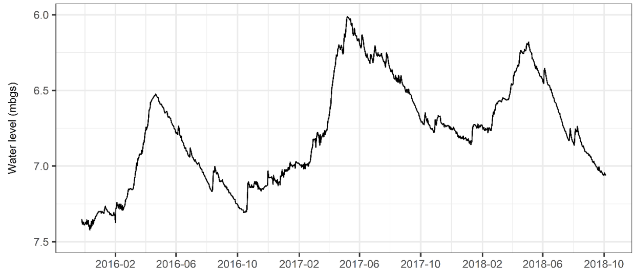
Fig. S2 Measured groundwater levels (depth below the ground surface) at the STEL site from 2016 to 2018
