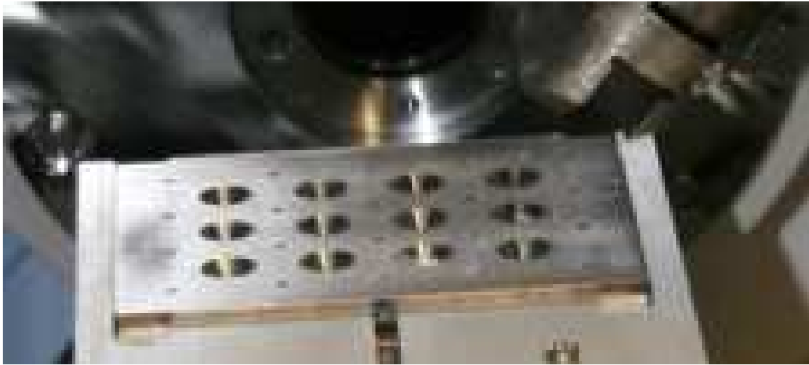
Photograph of aluminum block with depressed cavities, which functioned as the sample holder
