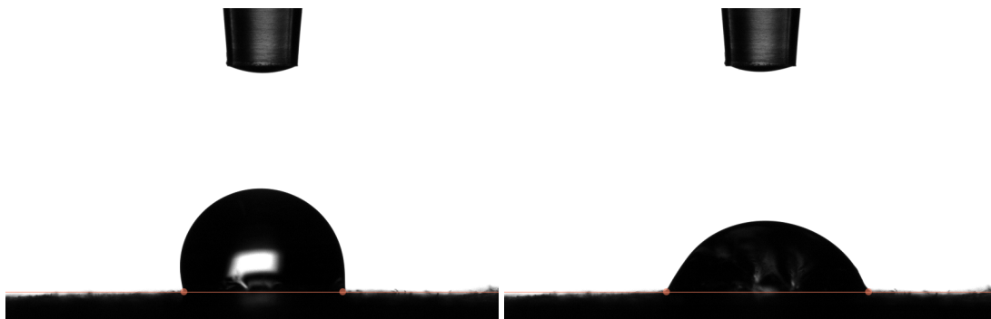
Figure S7: Water test CA on Foam-MC. The drop on the left side shows the initial CA after two seconds, and the drop on the right shows the CA after 20 s.
