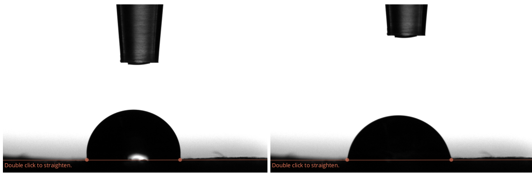
Figure S9: Water test CA on Foam-LN. The drop on the left side shows the initial CA after two seconds, and the drop on the right shows the CA after 20 s.
