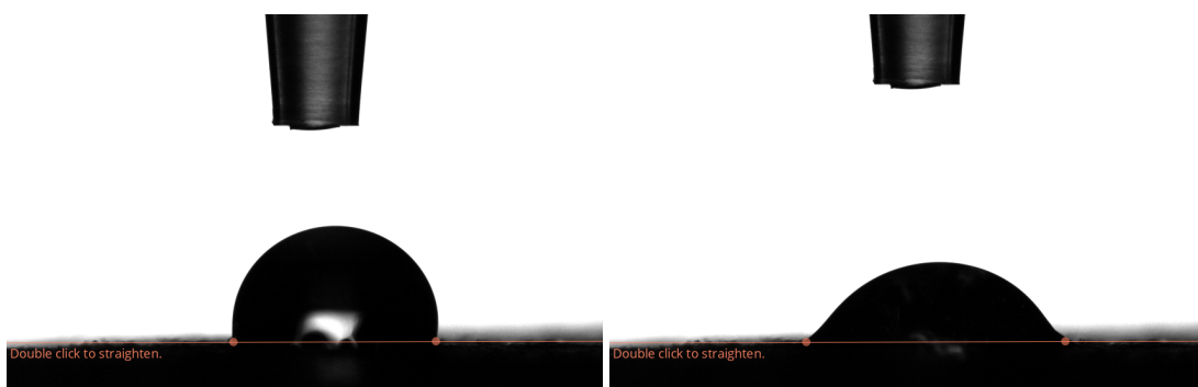
Figure S8: Water test CA on Foam-CF. The drop on the left side shows the initial CA after two seconds, and the drop on the right shows the CA after 20 s.
