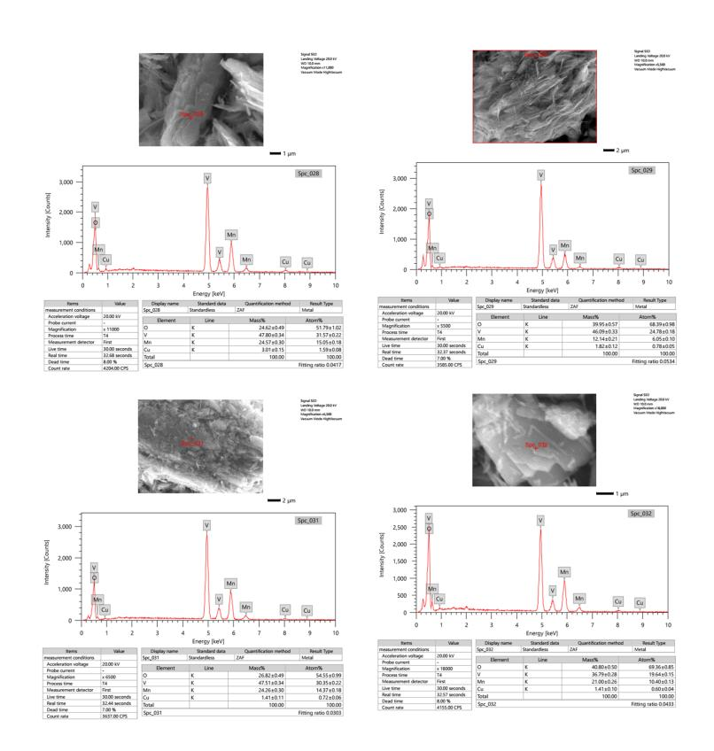
Figure S3. Replicas of EDX scans for cMCV6 at 4 different spots.
