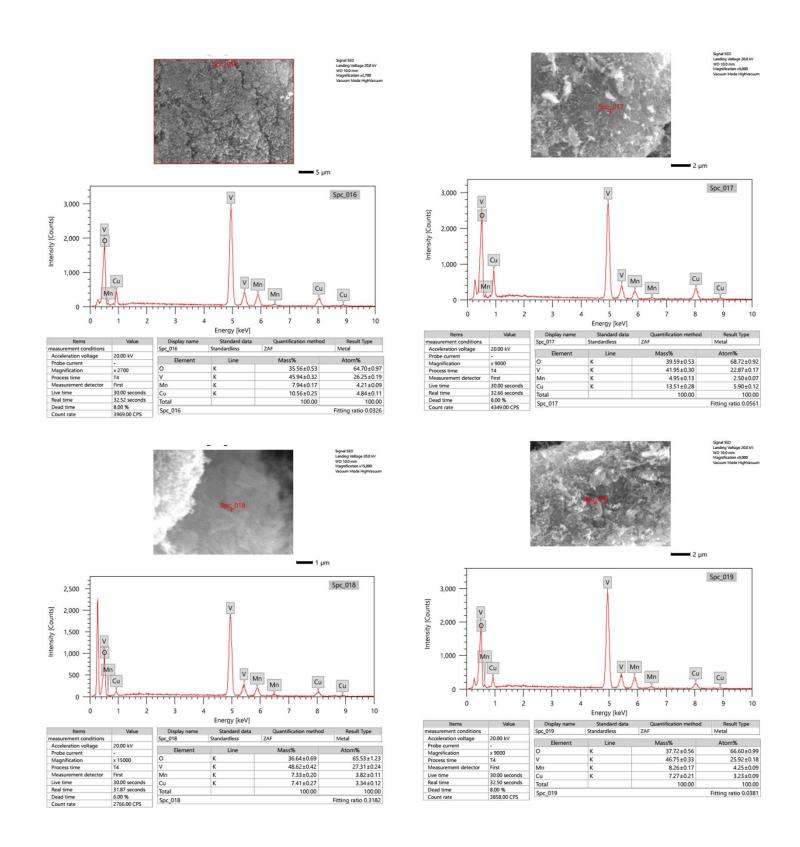
Figure S2. Replicas of EDX scans for cMCV4 at 4 different spots.
