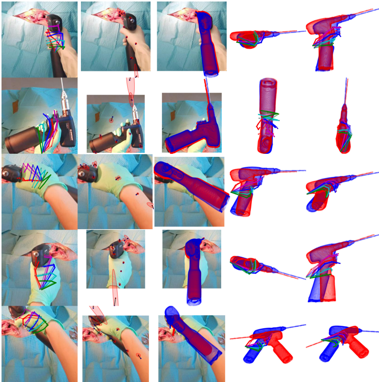
Fig. 4 Qualitative results of our proposed model on the real test data. The first column shows the estimated hand pose along with the transparent ground truth. In the second column, the estimated 2D keypoints are displayed in red, along with their 1\sigma standard deviation. Each line connects a keypoint estimate to the projection of the corresponding ground truth 3D keypoint. The third column visualizes 2D projections of the ground truth vertices in blue, and the predicted vertices in red. The last two columns display the 3D scene’s XZ and YZ subspace and correspond to views from the top and right, respectively. Note that the 3D views are not perspective views, nor was a z-buffer used to compute the correct occlusions.
