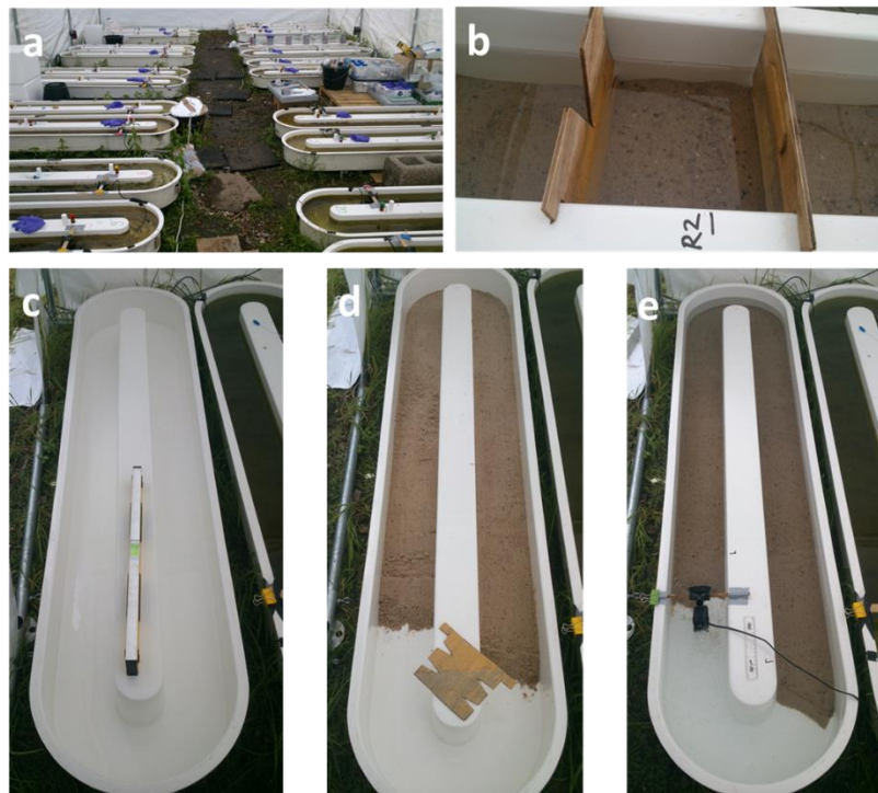
Figure S1.1: Pictures of the flume experiment. (a) overview of all flumes on day 47; (b) formation of bedforms using wooden plates; (c) leveling of an empty flume; (d) flume after filling and leveling the sediment; (e) flume after filling the water and installing the pump.
