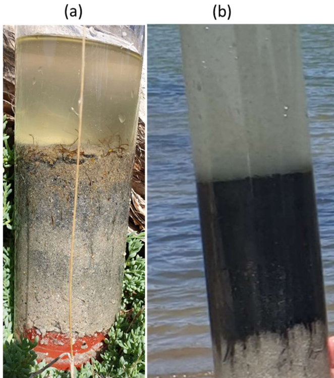
34 Examples of core samples from (a) Tea Tree and (b) Parnka Point taken with the polycarbonate push tube for analysis
